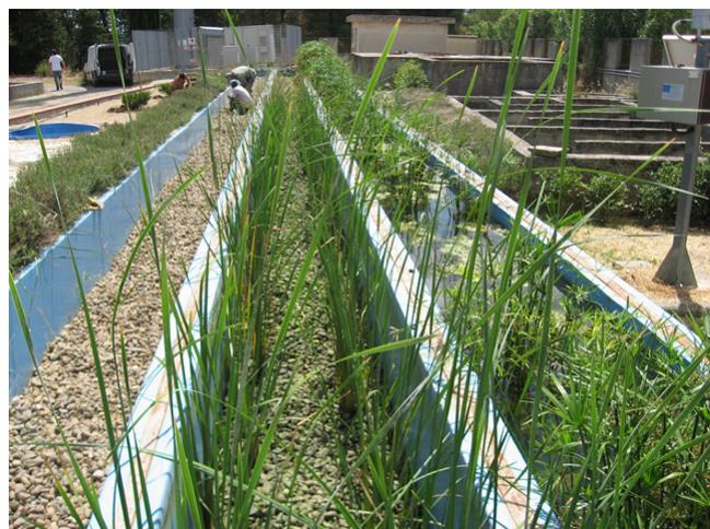
Fig. 1. A view of pilot-scale HSSF system located in Piana degli Albanesi (Sicily, Italy).
