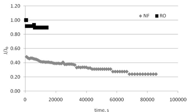
Fig. 5. Changes in relative permeate flux during the NF-90 and RO of geothermal water from Uniejow PIG/AGH-2.
