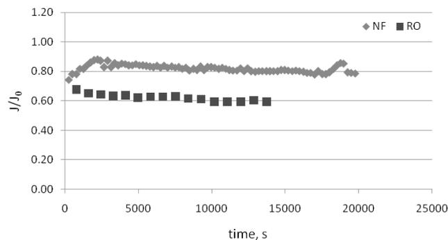
Fig. 4. Changes of relative permeate flux during the NF-270 and RO of geothermal water from Uniejow PIG/AGH-2.
