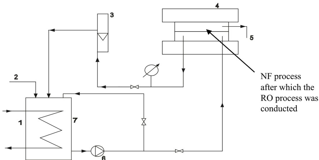
Fig. 1. Diagram of the apparatus for carrying out nanofiltration and reverse osmosis experiments in “cross-flow” mode (1-heat exchanger; 2-raw water inflow; 3-rotameter; 4-membrane cell; 5-permeate outflow; 6-pump; 7-raw water tank).
