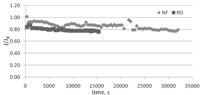
Fig. 3. Changes of relative permeate flux during the NF-270 and RO of Banska PGP-1 geothermal water.
