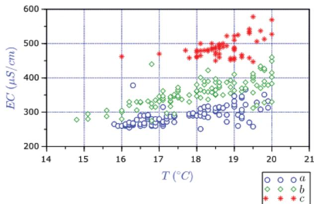
Fig. 6. Permeate conductivity during the Testing stage. Comparing permeates conductivity (EC) with TDS [9] we have the following intervals:
