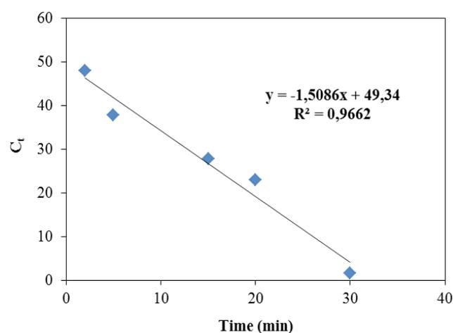
Fig. 9. Linearized zero-order kinetic plot for the decolorization of RY15 by Fenton oxidation.
