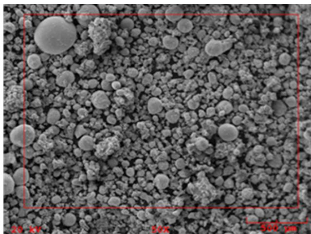
Fig. 1. SEM image of 8.0 wt.% Fe/CuO catalyst (magnification 50X).
