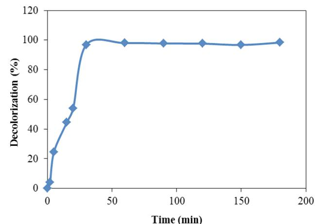
Fig. 8. Effect of reaction time on the decolorization of RY15 ([RY15] 50 mg/L,  $[H_2O_2] = 50$  mM, dosage of catalyst = 4.0 g/L with 8.0 wt.% of Fe/CuO, pH = 2, temperature = 30°C, and stirring speed = 140 rpm).
