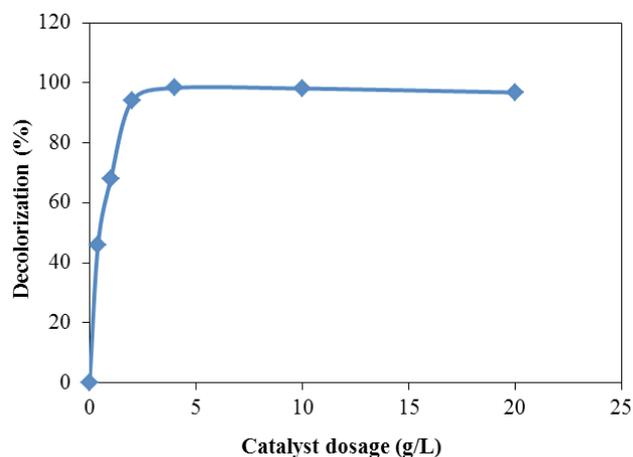
Fig. 3. Effect of dosage of catalyst on the decolorization of RY15 ([RY15] = 50 mg/L,  $[\text{H}_2\text{O}_2]$  = 50 mM, 8.0 wt.% of Fe/CuO,  $\text{pH} = 2$ , time = 180 min, temperature = 30°C, and stirring speed = 140 rpm).
