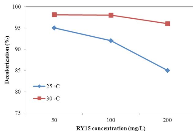
Fig. 7. Effect of initial dye concentration on the decolorization of RY15 ( $[\text{H}_2\text{O}_2]$  = 50 mM, dosage of catalyst = 4.0 g/L with 8.0 wt.% of Fe/CuO, pH = 2, time = 60 min, temperature = 30°C, and stirring speed = 140 rpm).
