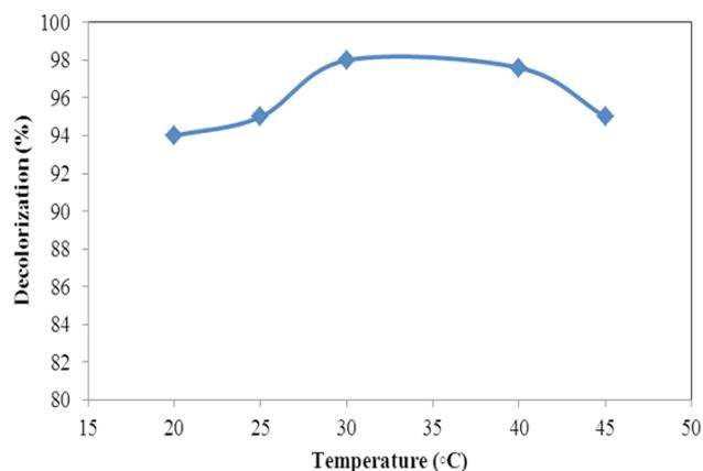
Fig. 5. Effect of temperature on the decolorization of RY15 ([RY15] = 50 mg/L,  $[\text{H}_2\text{O}_2]$  = 50 mM, dosage of catalyst = 4.0 g/L with 8.0 wt.% of Fe/CuO,  $\text{pH} = 2$ , time = 60 min, and stirring speed = 140 rpm).
