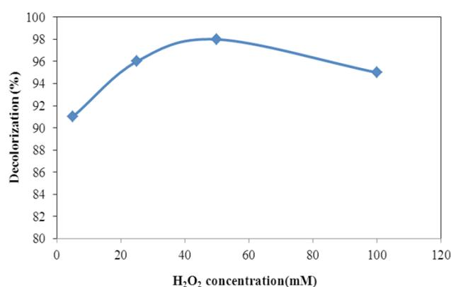
Fig. 6. Effect of  $\text{H}_2\text{O}_2$  concentration on the decolorization of RY15 ([RY15] = 50 mg/L, dosage of catalyst = 4.0 g/L with 8.0 wt.% of Fe/CuO, pH = 2, time = 60 min, temperature = 30°C, and stirring speed = 140 rpm).
