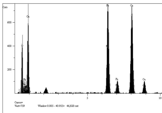
Fig. 2. EDX spectra of 8.0 wt.% Fe/CuO catalyst.
