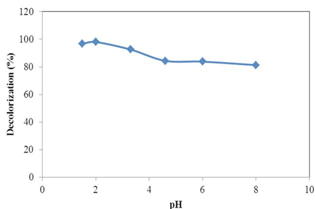
Fig. 4. Effect of pH on the decolorization of RY15 ([RY15] = 50 mg/L,  $[\text{H}_2\text{O}_2]$  = 50 mM, dosage of catalyst = 4.0 g/L with 8.0 wt.% of Fe/CuO, time = 60 min, temperature = 30°C, and stirring speed = 140 rpm).
