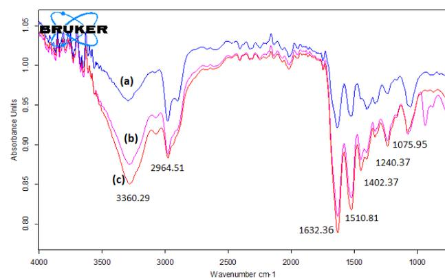
Fig. 4. FT-IR spectra (a) GL-HFO, (b) GL/Cr(VI), (c) GL.
