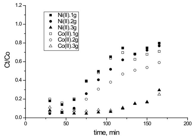
Fig. 5. Effect of resin load on Ni(II) and Co(II) adsorption (initial ion concentration 0.01 g/L, pH = 3.1, flow rate 6 cm<sup>3</sup>/min).
