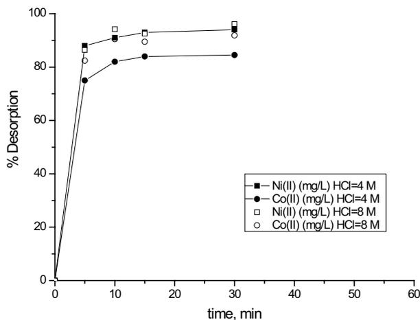
Fig. 3. Desorption of Ni(II) and Co(II) from the resin (load 1 g) by HCl at different concentrations (4 and 8 M; volume of 20 mL).
