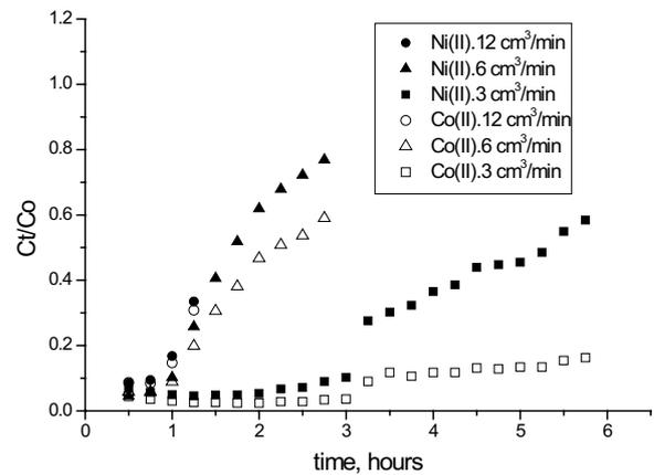
Fig. 4. Effect of flow rate on Ni(II) and Co(II) adsorption over time (initial ion concentration 0.01 g/L, pH = 3.1, resin load 2 g).
