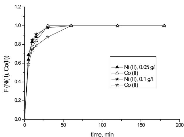
Fig. 2. Effect of the initial Ni(II) and Co(II) concentration (0.05 and 0.1 g/L) on the value of  $F$  at different extraction times, at a pH of 3.1 and for a 2-g resin load.
