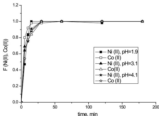
Fig. 1. Effect of pH on the value of  $F$  for Ni(II) and Co(II) at different extraction times, for a concentration of 0.05 g/L ions, and for a 2-g resin load.
