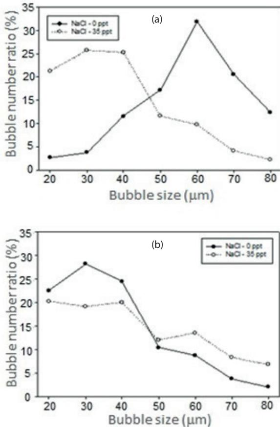
Fig. 3. Bubble size distribution under air at: (a) 2 atm and (b) 5 atm.
