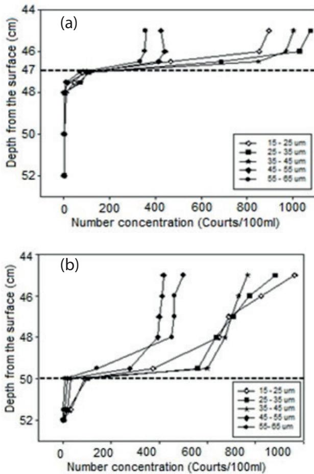
Fig. 5. Bubble bed depth under air at 5 atm with: (a) NaCl 0 ppt and (b) NaCl 35 ppt.
