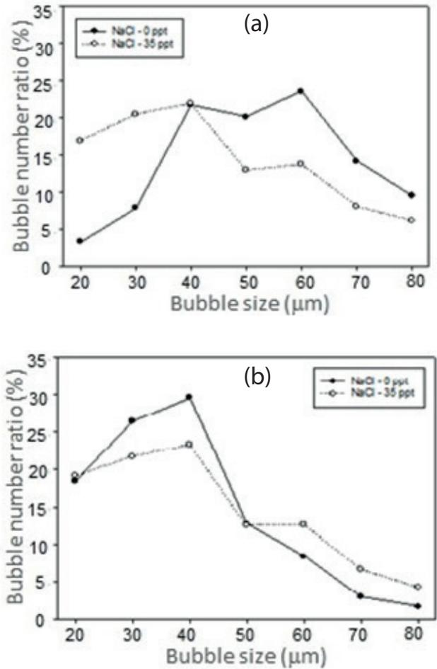
Fig. 4. Bubble size distribution under CO<sub>2</sub> at: (a) 2 atm and (b) 5 atm.
