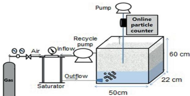
Fig. 1. Schematic diagram of the bubble size measurement apparatus.
