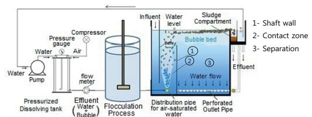
Fig. 2. Schematic diagram of the pilot plant.
