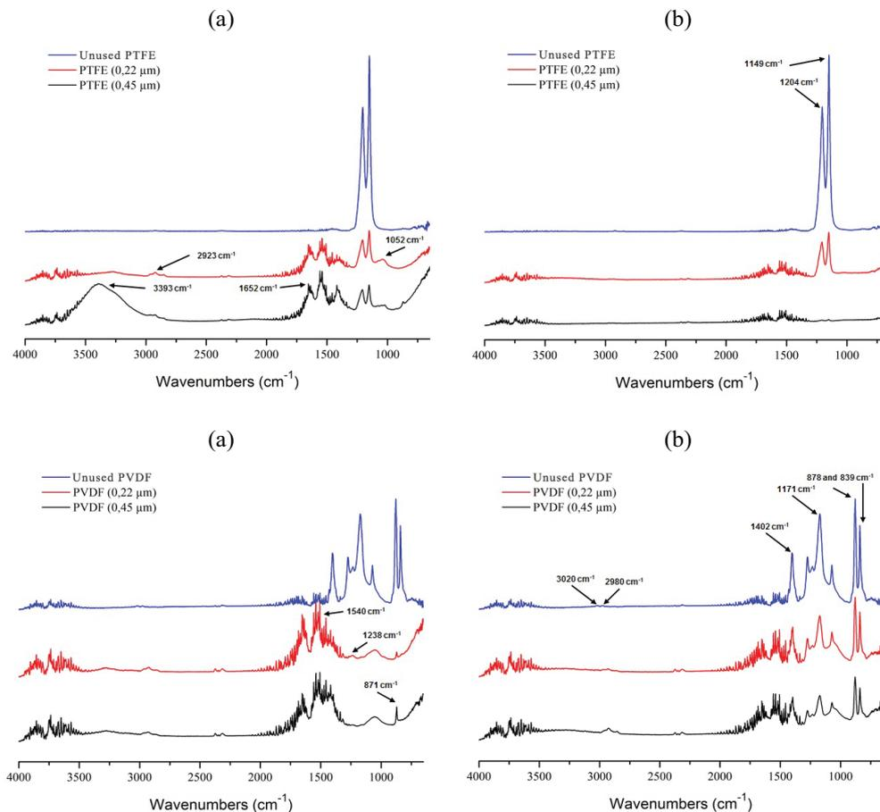
Fig. 5. FTIR spectra of PTFE and PVDF membranes before and after MD process: (a) raw leachate and (b) pretreated leachate.
