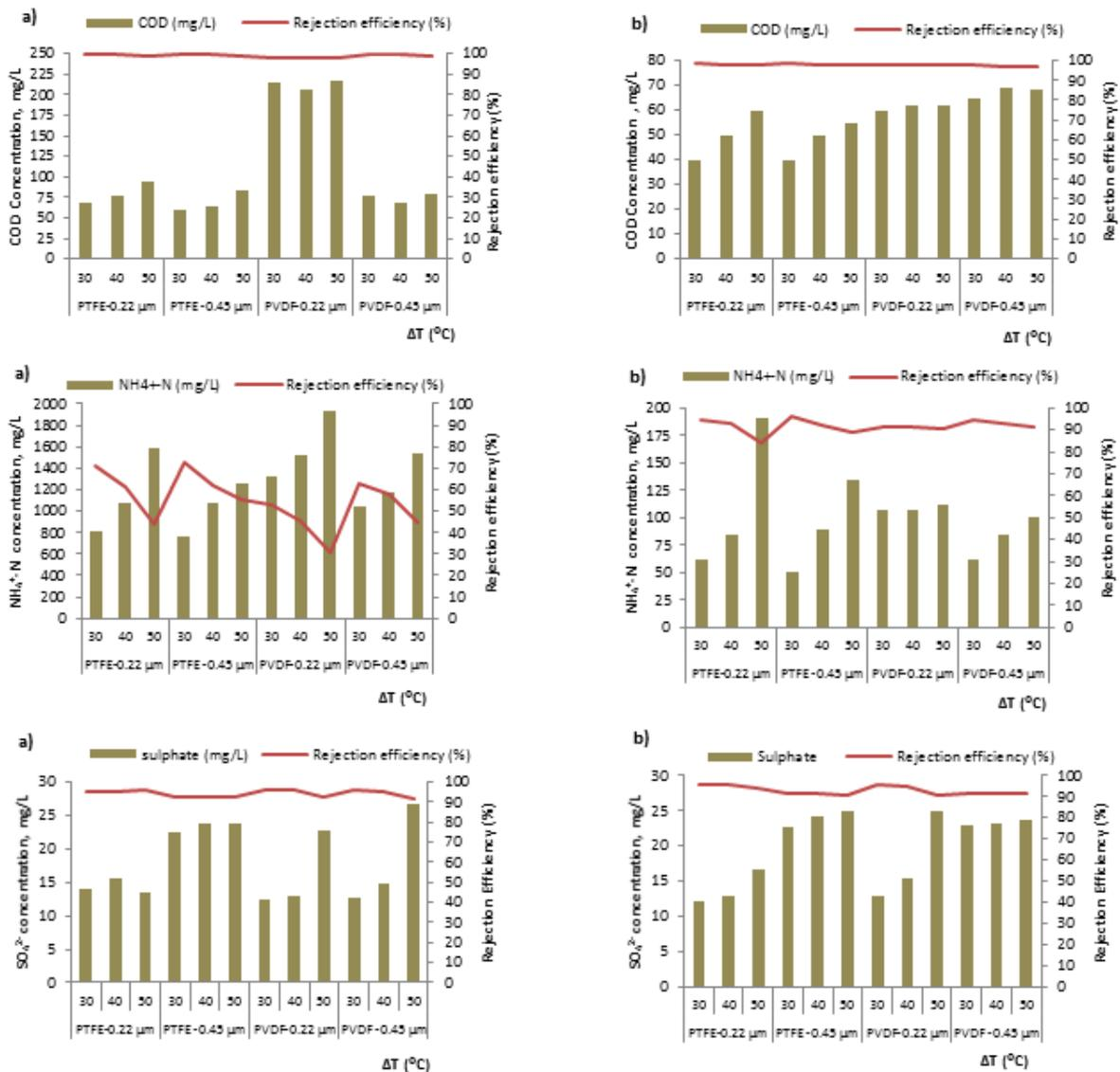
Fig. 3. COD,  $\text{NH}_4^+-\text{N}$  and  $\text{SO}_4^{2-}$  concentration of permeate from various membranes at three different  $\Delta T$ : (a) raw leachate and (b) pretreated leachate.
