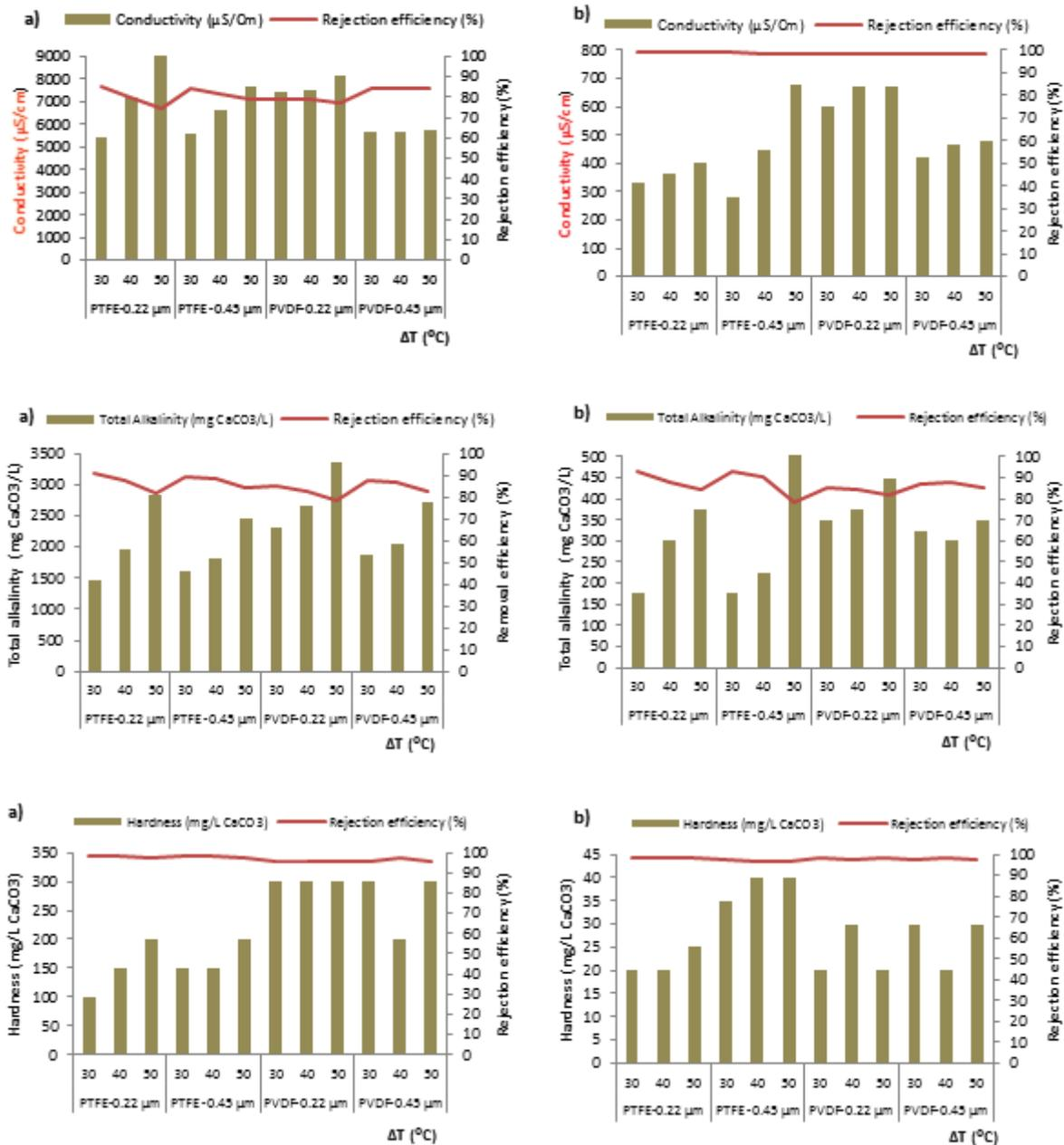
Fig. 2. Conductivity, total alkalinity and hardness of permeate water from various membranes at three different  $\Delta T$  (30°C, 40°C and 50°C): (a) raw leachate and (b) pretreated leachate.
