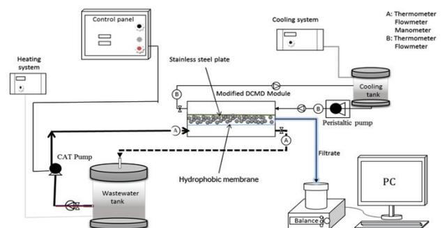
Fig. 1. Schematic flow diagram of the lab-scale modified DCMD.
