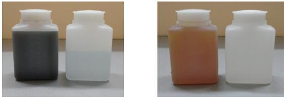
Fig. S1. (a) Raw landfill leachate (left) and permeate from MD (right), and (b) pretreated landfill leachate (left) and permeate from MD (right).
