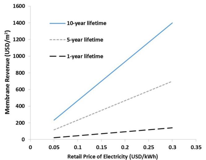
Fig. 4. Economic analysis for membrane revenue per surface area of the membrane as a function of the average retail price of electricity and durability of a membrane (lifetime) for the ZarrinehRud River.
