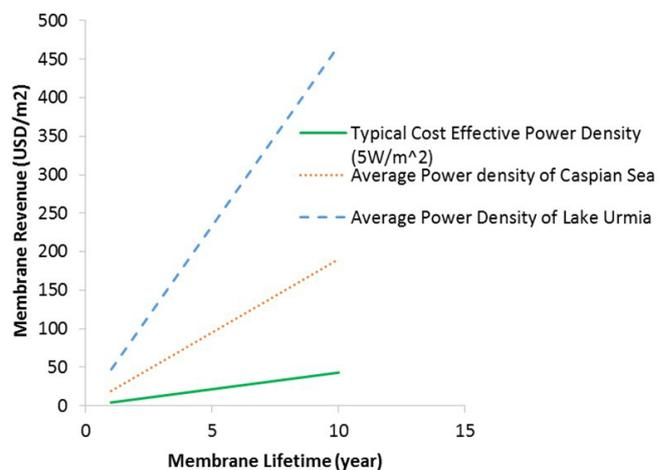
Fig. 5. Economic analysis for membrane revenue per surface area of the membrane as a function of membrane lifetime.
