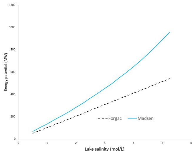
Fig. 2. A comparison of mixing energy potential of Urmia Lake between two presented models of Madsen et al. [11] and Forgacs [21].
