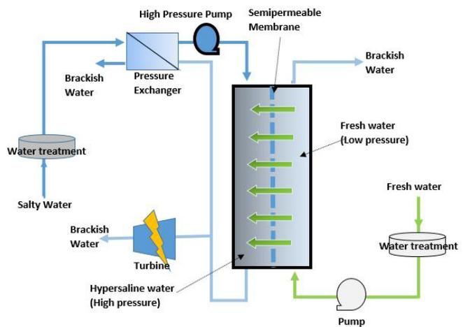
Fig. 3. Schematic diagram of a typical PRO power plant with counter current flow at steady-state condition.
