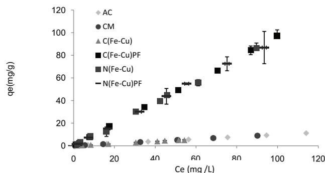
Fig. 11. Adsorption isotherms of phenol at 50°C.
