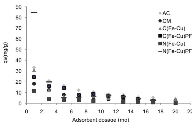
Fig. 10. Adsorbent dosages vs. adsorption capacities of phenol.
