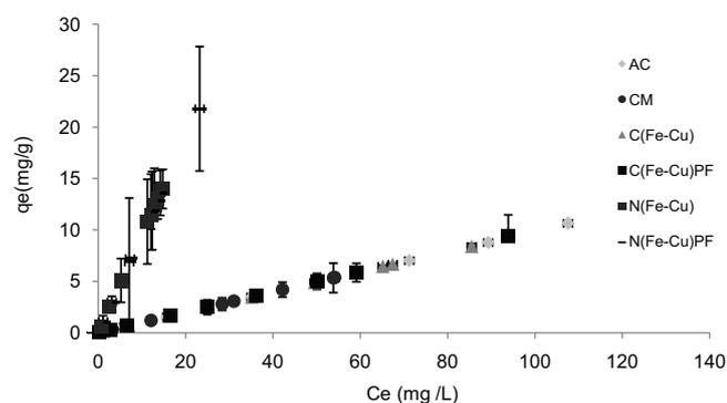
Fig. 8. Adsorption isotherms of phenol at 30°C.
