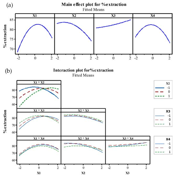
Fig. 4. Plot of the effect of pH effects of feed solution ( $X_1$ ), (+)-DBTA ( $X_2$ ) concentration, Temperature ( $X_3$ ), and flow rates of feed and stripping solutions ( $X_4$ ) on the extraction of (S)-amlodipine. (4a) the main effect plots and (4b) the interaction plots.
