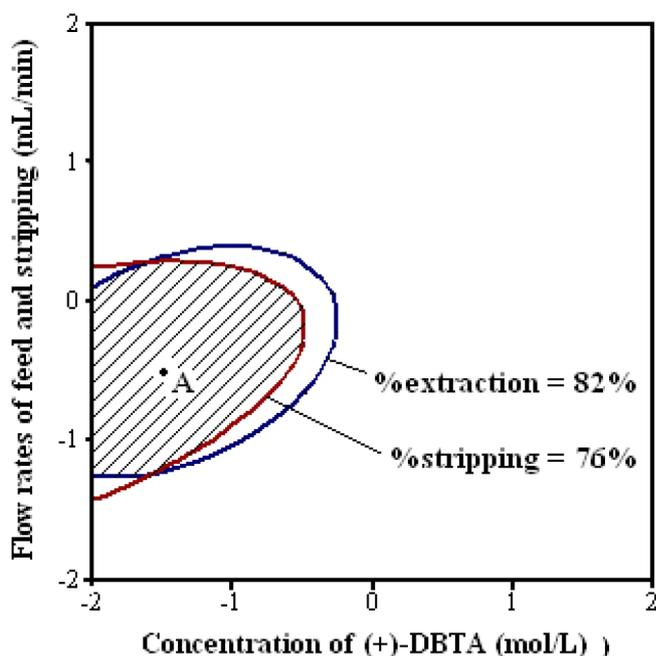
Fig. 7. Superimposed contour plots showing the shaded overlapping area for which %extraction  $\geq$  82% and %stripping  $\geq$  76%.
