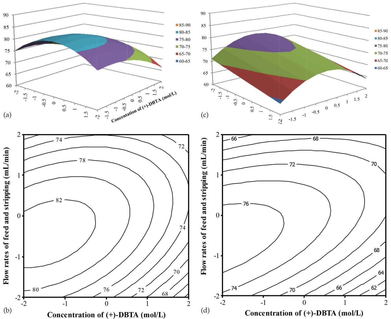
Fig. 6. Contour plots showing the effect of concentration of (+)-DBTA ( $X_2$ ) and flow rates of feed and stripping solutions ( $X_4$ ) and stripping (6b) of (S)-amlodipine. (6a) Response surface of extraction, (6b) Contour plot of extraction, (6c) Response surface of stripping, (6d) Contour plot of stripping.
