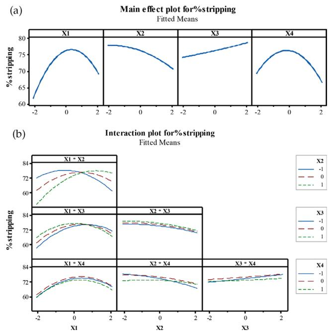
Fig. 5. Plot of the effect pH effects of feed solution ( $X_1$ ), (+)-DBTA ( $X_2$ ) concentration, Temperature ( $X_3$ ), and flow rates of feed and stripping solutions ( $X_4$ ) on stripping of (S)-amlodipine. (5a) the main effect plots and (5b) the interaction plots.
