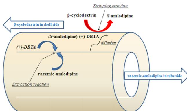
Fig. 2. Transport scheme for chiral extraction.
