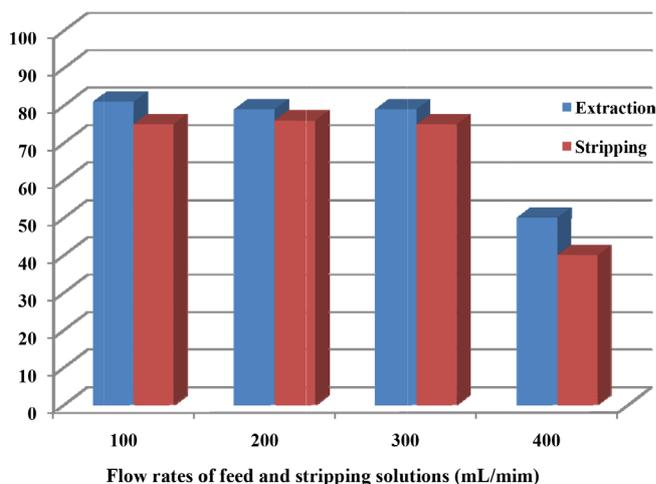
Fig. 8. The relation between flow rates and percentages of extraction and stripping.
