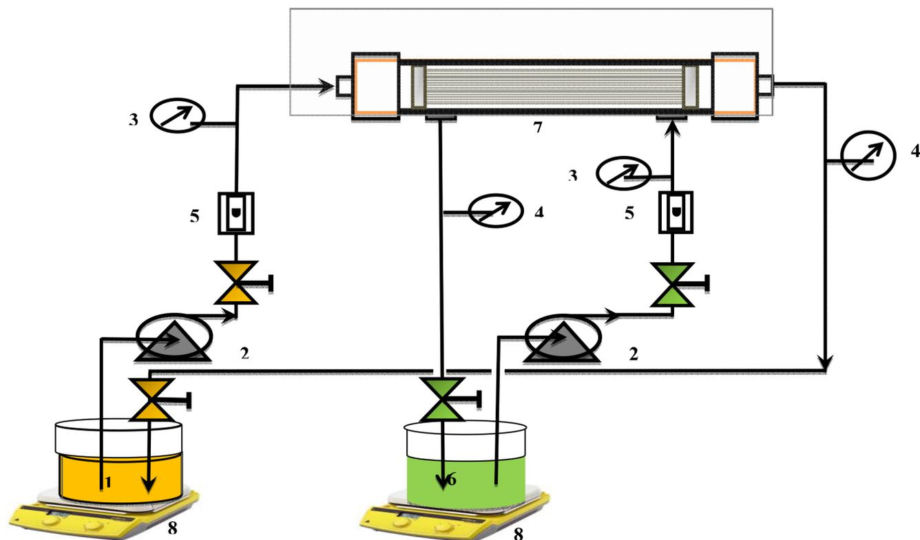
Fig. 3. Schematic counter-current flow diagram for circulated mode operation of a hollow fiber supported liquid membrane system. 1. Feed solution tank 2. Gear pump 3. Inlet pressure gauges 4. Outlet pressure gauges 5. Flow meters 6. Stripping solution tank 7. Hollow fiber module 8. heater.
