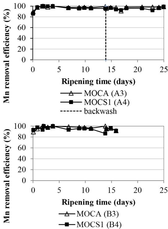
Fig. 6. Mn removal efficiency (%) as a function of the filter run time for pilot filters containing a layer of fresh MOCS<sub>1</sub> or MOCA; feed water without (left) and with UF (right) pre-treatment.
