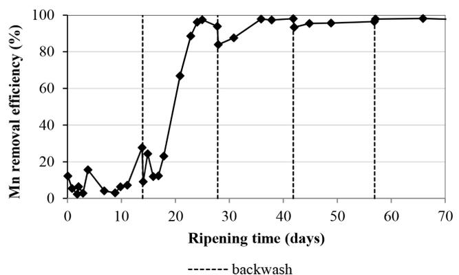
Fig. 4. Effect of filter backwashing on manganese removal efficiency during filter media ripening with virgin sand.
