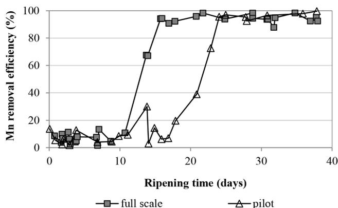
Fig. 5. Comparison of the Mn removal efficiency as a function of the filter ripening time for full scale and pilot filters with virgin anthracite (filtration rate:  $V_f = 5.1$  m/h pilot filter and  $V_f = 2.5$  m/h full scale filter).
