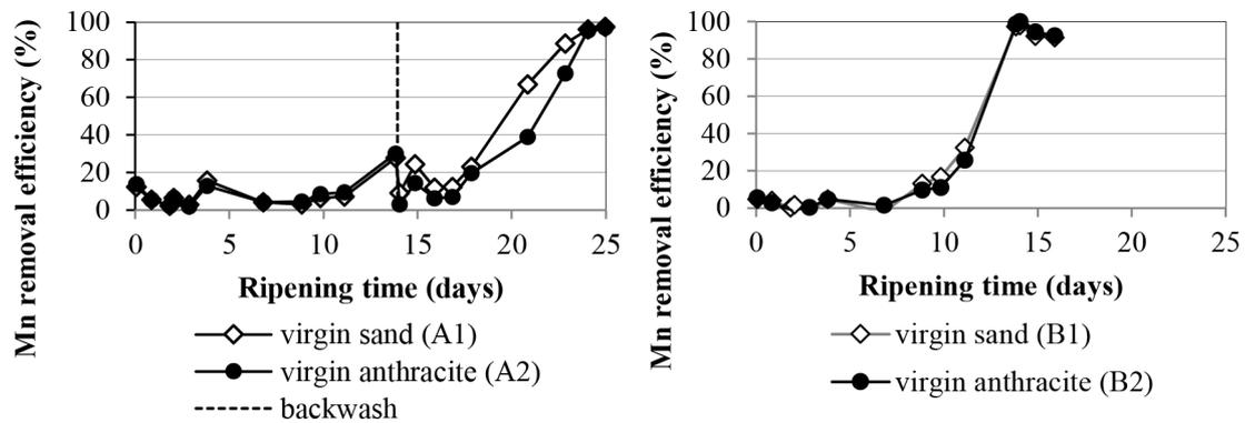
Fig. 3. Mn removal efficiency (%) as a function of the filter ripening time, type of virgin filter media and UF pre-treatment; feed water without (left), and with UF pre-treatment (right).
