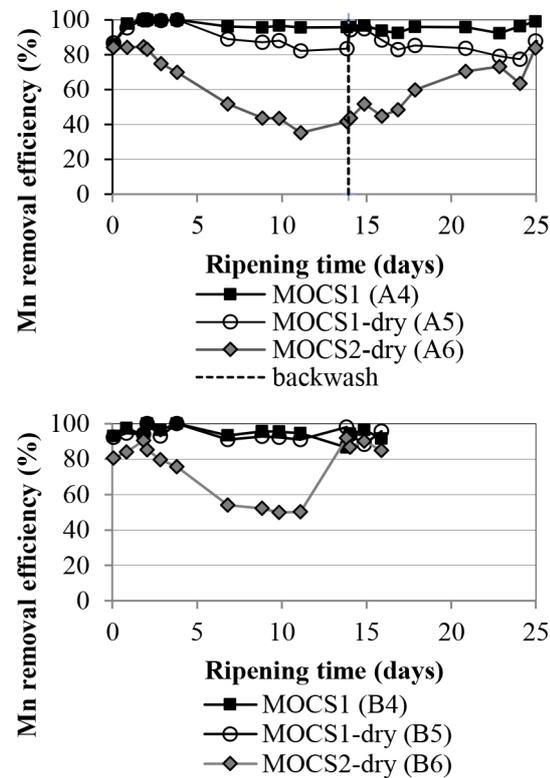
Fig. 7. The Mn removal efficiency as a function of filter run time for pilot filters containing layers of dried or fresh MOCS; feed water without (left) and with UF (right) pre-treatment.
