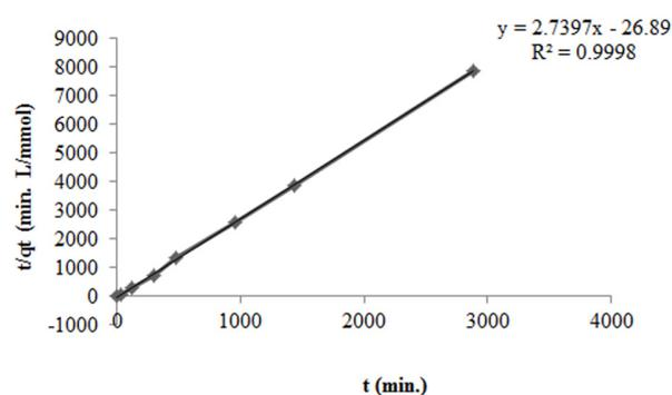
Fig. 10. The fitting of pseudo-second-order model for Cr(III) on PSF/TTU microcapsule (Cr(III): 50 mg/L, adsorbent amount: 0.05 g, pH: 5, temperature: 298 K).
