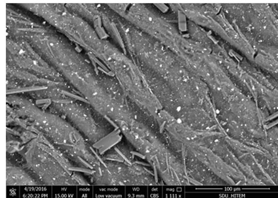
Fig. 4. SEM image of PSF/TTU microcapsule.
