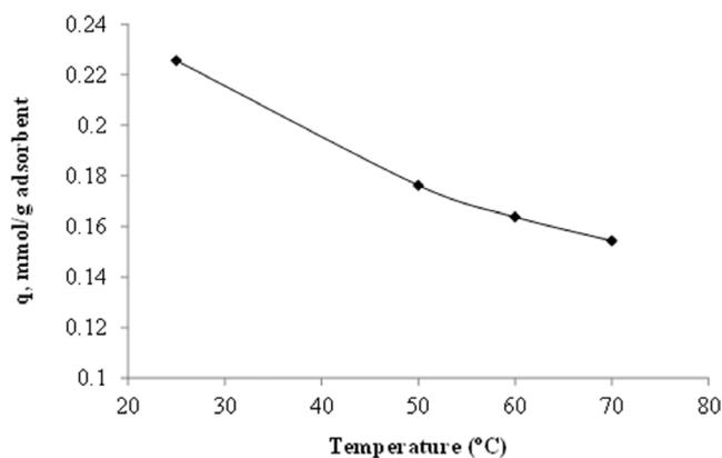
Fig. 12. The effect of temperature on the adsorption of Cr(III) (Cr(III): 50 mg/L, adsorbent amount: 0.05 g, pH: 5, t: 5 h).
