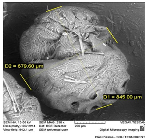
Fig. 5. SEM image of PSF/TTU microcapsule.
