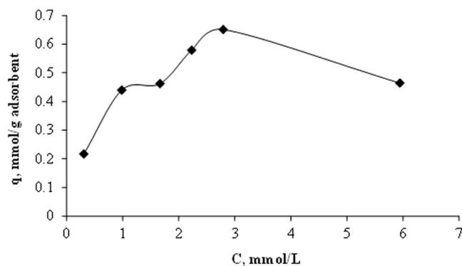
Fig. 13. The effect of initial concentration on the adsorption of Cr(III) (Adsorbent amount: 0.05 g, pH:5, t: 5 h, temperature: 298 K).
