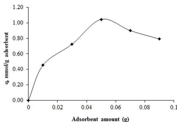
Fig. 11. The effect of adsorbent amount on the adsorption of Cr(III) (Cr(III): 50 mg/L, pH:5, t: 5 h, temperature: 298 K).
