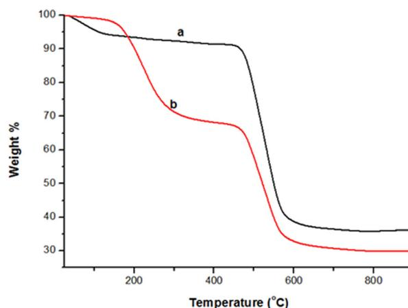
Fig. 7. Thermogravimetric diagrams of (a) PSF, (b) PSF/TTU microcapsule.
