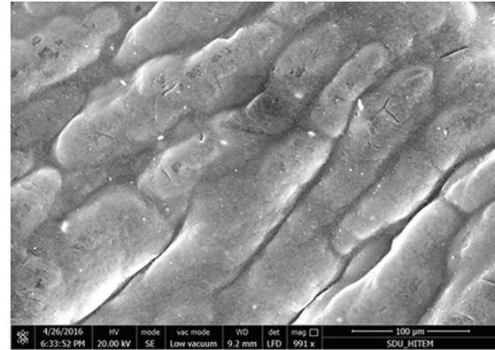
Fig. 3. SEM image of original PSF microcapsule.
