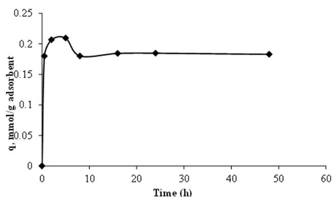
Fig. 9. The effect of time on the adsorption of Cr(III) (Cr(III): 50 mg/L, adsorbent amount: 0.05 g, pH: 5, temperature: 298 K).
