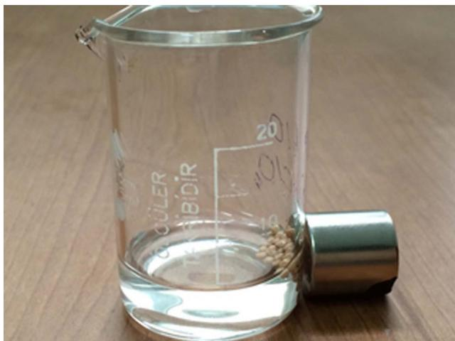
Fig. 2. Photograph of PSF/TTU microcapsules attracted by a magnet.
