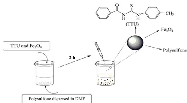
Fig. 1. Schematic procedure of magnetic PSF/TTU microcapsule production.
