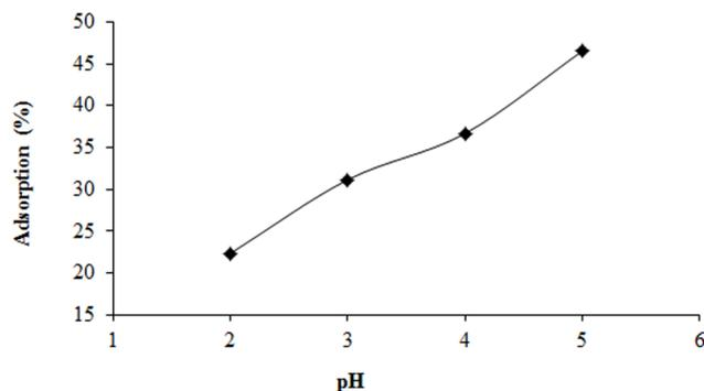
Fig. 8. The effect of pH on the adsorption of Cr(III) (Cr(III): 50 mg/L, adsorbent amount: 0.05 g,  $t$ : 5 h, temperature: 298 K).
