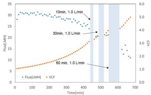
Fig. 6. Flux and VCF at 1.0 L/min of acid cleaning test.
