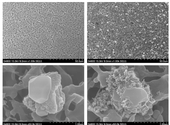
Fig. 7. Scanning electron microscope pictures for crystals on the membrane surface: (a) flow rate at 0.2 L/min and (b) flow rate at 1.0 L/min.
