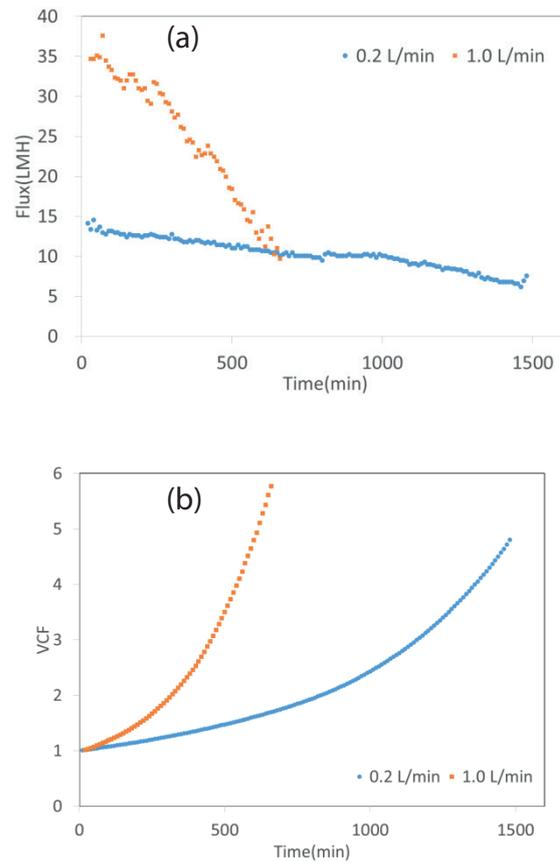
Fig. 3. Flux and VCF of MD flow velocity (no cleaning). (a) Flux of MD flow velocity and (b) VCF of MD flow velocity.
