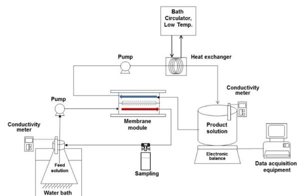
Fig. 1. Schematics of DCMD operation.
