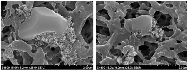
Fig. 8. Scanning electron microscope pictures for crystals on the membrane surface after cleaning: (a) flow rate at 0.2 L/min and (b) flow rate at 1.0 L/min.
