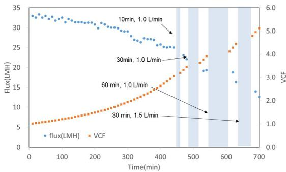
Fig. 5. Flux and VCF at 1.0 L/min of deionized water cleaning test.
