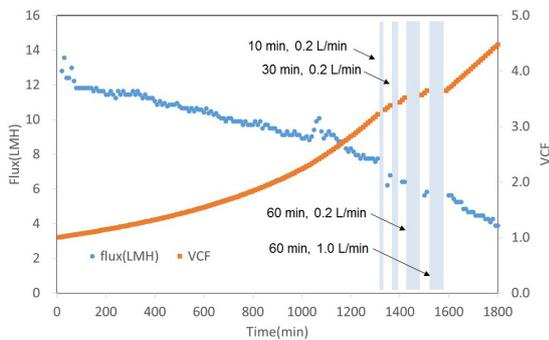
Fig. 4. Flux and VCF at 0.2 L/min of deionized water cleaning test.
