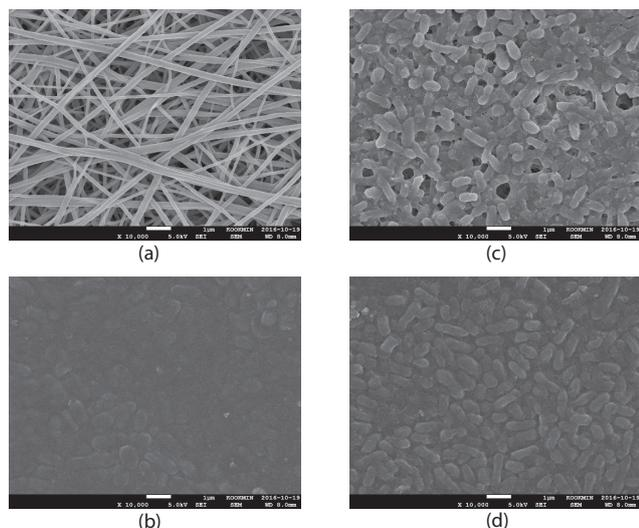
Fig. 6. SEM images for electrospun membranes (magnification: 10,000 times): (a) original membrane; (b) without pretreatment (raw water, sample 1); (c) pretreatment using coagulation at PAC dose 557 mg/L, pH 11.2, and temperature 65.2°C (sample 2); and (d) pretreatment using coagulation at PAC dose 1,094 mg/L, pH 2.8, and temperature 29°C (sample 3).
