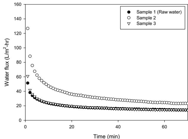
Fig. 5. Effect of coagulation pretreatment on permeate flux in MF.
