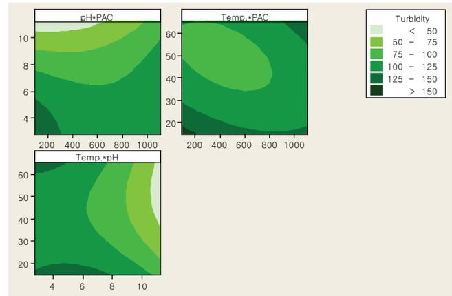
Fig. 1. Response surface of the effects of two independent variables for turbidity,  $Y_1$ .
