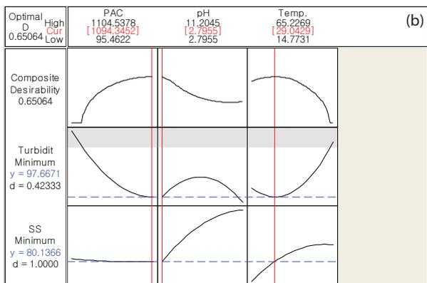
Fig. 4. Optimization of coagulation conditions using response optimization method: (a) the optimal condition for the turbidity, SS, and COD to the minimum and (b) the optimal condition for the turbidity and SS to the minimum.
