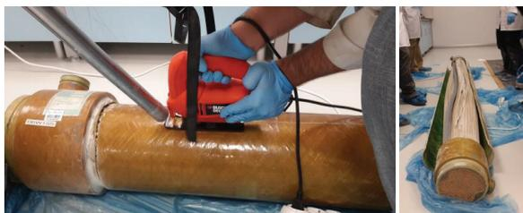
Fig. 2. Dismounting of the membrane module vessel.
