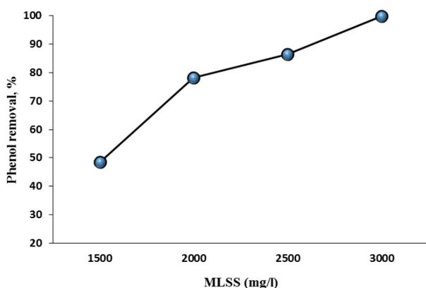
Fig. 5. Phenol removal efficiency at various concentrations of MLSS (initial increasing phenol concentration of 500 mg/L).
