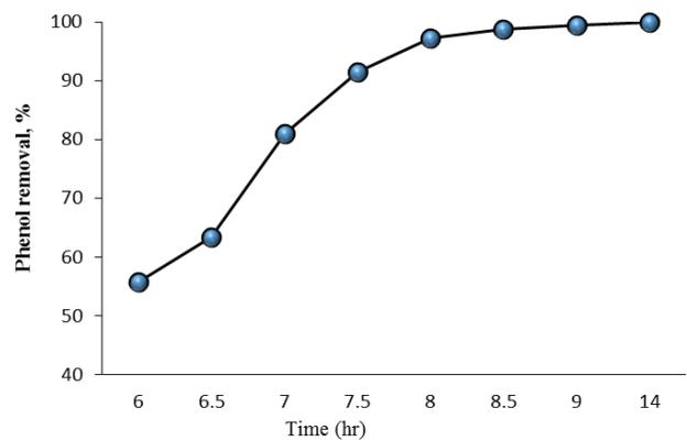
Fig. 4. Phenol removal efficiency at various residence times for phenol removal from aqueous solutions (initial phenol concentration of 500 mg/L, and glucose increasing concentration of 250 mg/L).
