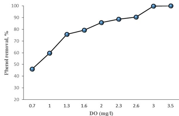
Fig. 6. Phenol removal efficiency at various dissolved oxygen concentrations for phenol removal from aqueous solutions (initial increasing phenol concentration of 500 mg/L).
