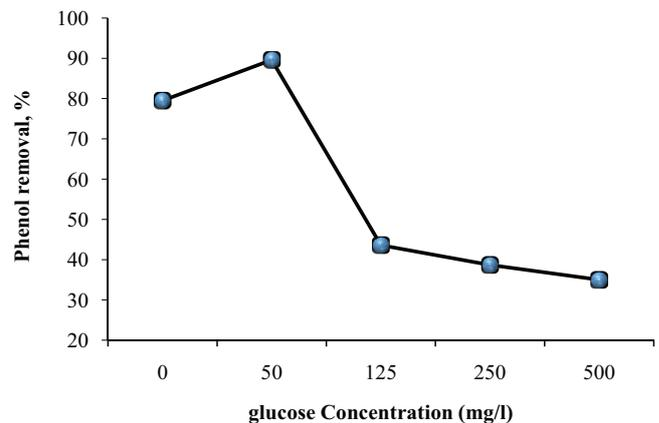
Fig. 2. Phenol removal efficiency at various glucose concentrations for phenol removal from aqueous solutions (initial phenol concentration of 500 mg/L).
