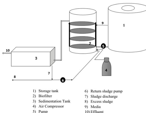
Fig. 1. Schematic of studied BF/AS combined system.
