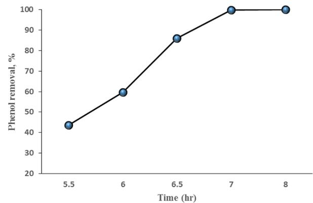
Fig. 3. Phenol removal efficiency at various residence times for phenol removal from aqueous solutions (initial phenol concentration of 500 mg/L).
