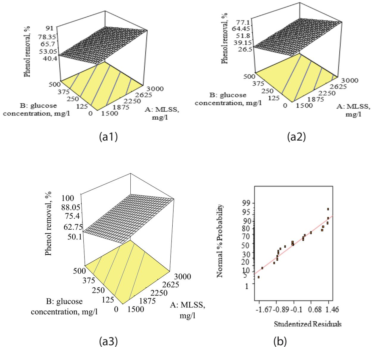
Fig. 7. Three-dimensional plan (a) interaction impact of MLSS concentration and glucose for phenol removal through BF/AS system and dissolved oxygen concentration (a1) 1 mg/L, (a2) 2 mg/L, (a3) 3 mg/L and (b) normal plot of residuals.
