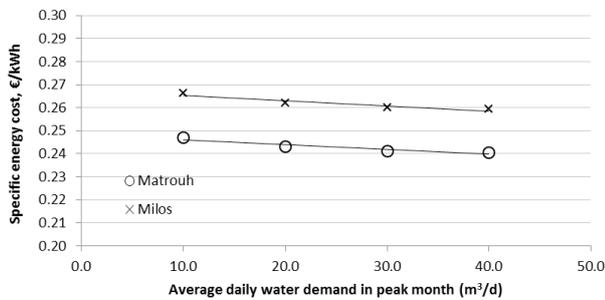
Fig. 8. Specific energy cost in €/kWh in the peak month for AC plants.
