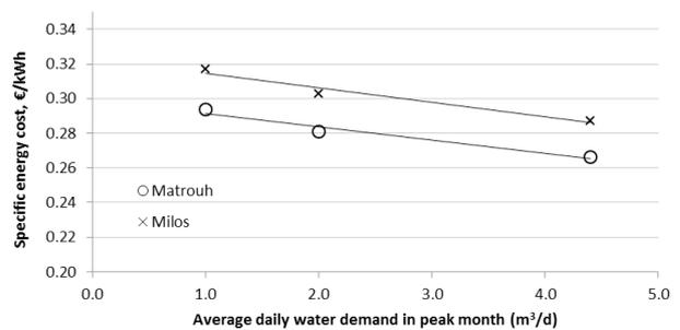
Fig. 7. Specific energy cost in €/kWh in the peak month for DC plants.
