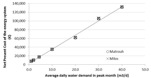
Fig. 6. Net present cost of the electrical energy producing subsystem for Matrouh and Milos.
