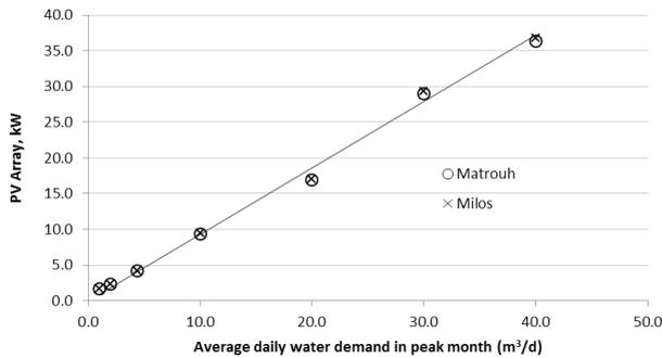
Fig. 4. The PV array size with the average daily water demand in the peak month.
