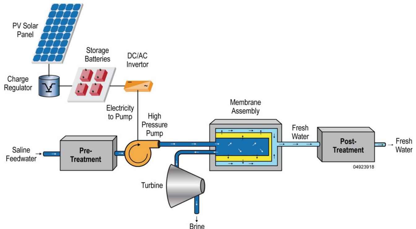
Fig. 1. Layout of a PV/RO system with energy recovery.
