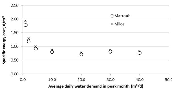
Fig. 9. Specific energy cost in €/m<sup>3</sup> in the peak month.
