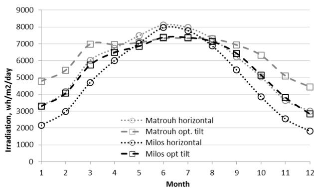
Fig. 3. Monthly average global irradiation on horizontal and optimally inclined planes at Matrouh and Milos.
