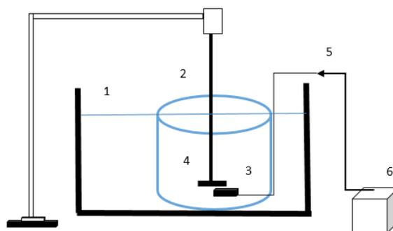
Fig. 1. Schematic of pilot study: 1 – ultrasonic chamber, 2 – reactor, 3 – mixer, 4 – mixer holder, 5 – air hose, and 6 – air pump.
