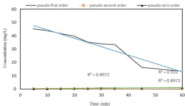
Fig. 6. Reaction kinetic of 2,4-DCP decomposition in US/ $\text{H}_2\text{O}_2$  process.
