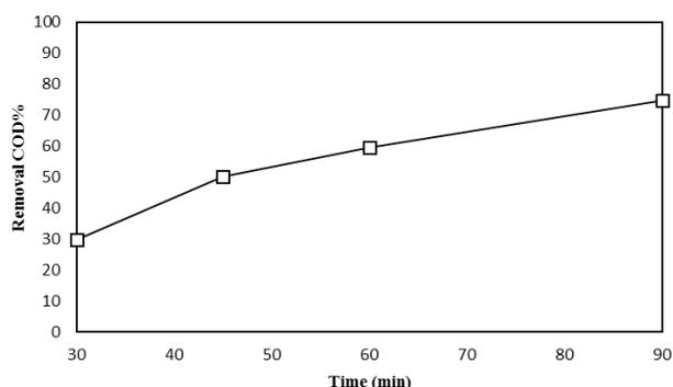
Fig. 7. Effect of US/H<sub>2</sub>O<sub>2</sub> process on COD removal (pH = 3 and DCP = 0.3 mol/L).
