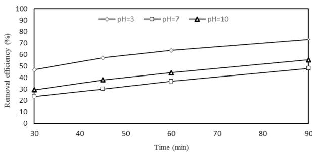
Fig. 2. Effect of pH on US/H<sub>2</sub>O<sub>2</sub> process efficiency in 2,4-DCP removal (H<sub>2</sub>O<sub>2</sub> = 0.08 mol/L and 2,4-DCP = 0.3 mol/L).
