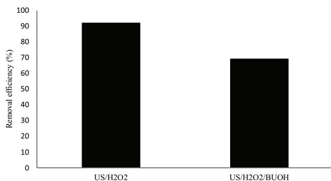
Fig. 4. Effect of *tert*-butanol on US/ $\text{H}_2\text{O}_2$  process under optimal conditions (reaction time = 90 min, pH = 3,  $\text{H}_2\text{O}_2$  concentration = 0.1 mol/L, and initial 2,4-DCP concentration = 0.3 mol/L).
