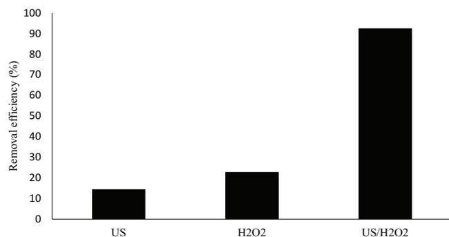
Fig. 5. Effect of US alone,  $\text{H}_2\text{O}_2$  alone, and US/ $\text{H}_2\text{O}_2$  on the oxidation of 2,4-DCP (optimal conditions obtained from previous steps: pH = 3,  $\text{H}_2\text{O}_2$  concentration = 0.1 mol/L, and 2,4-DCP = 0.3 mol/L).
