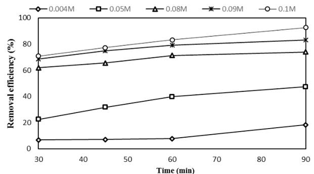
Fig. 3. Effect of H<sub>2</sub>O<sub>2</sub> concentration on US/H<sub>2</sub>O<sub>2</sub> process efficiency in 2,4-DCP removal (pH = 3 and 2,4-DCP = 0.3 mol/L).
