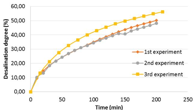
Fig. 6. Desalination degree evolution during three experiments (percentage expression of the amount of salts that can be removed by one passage during the electro dialysis process at given linear flow rate and inlet salt concentration).
