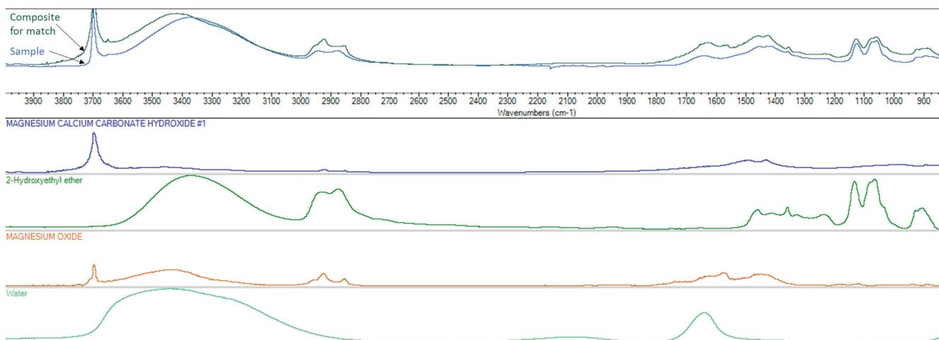
Fig. 5. FTIR spectrum of the clogging film.
