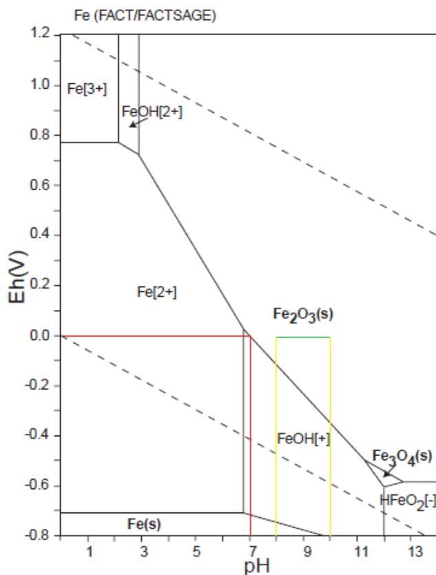
Fig. 2. Pourbaix diagram for iron. Optimum pH for precipitation is between 8 and 10.
