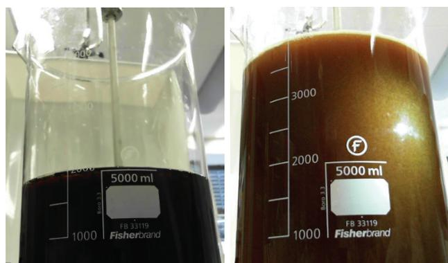
Fig. 1. Coagulation of 2.2 L of DEG with 2.2 L of demineralized water by organic agent before (left) and after (right) addition of water and chemicals.
