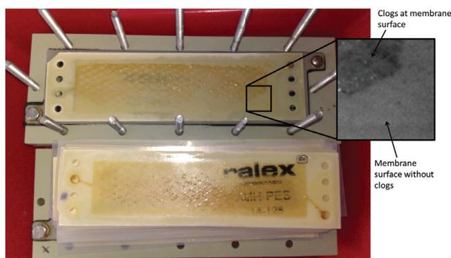
Fig. 4. Disassembled ED module. Clogs at membrane surface are highlighted by grayscale image.
