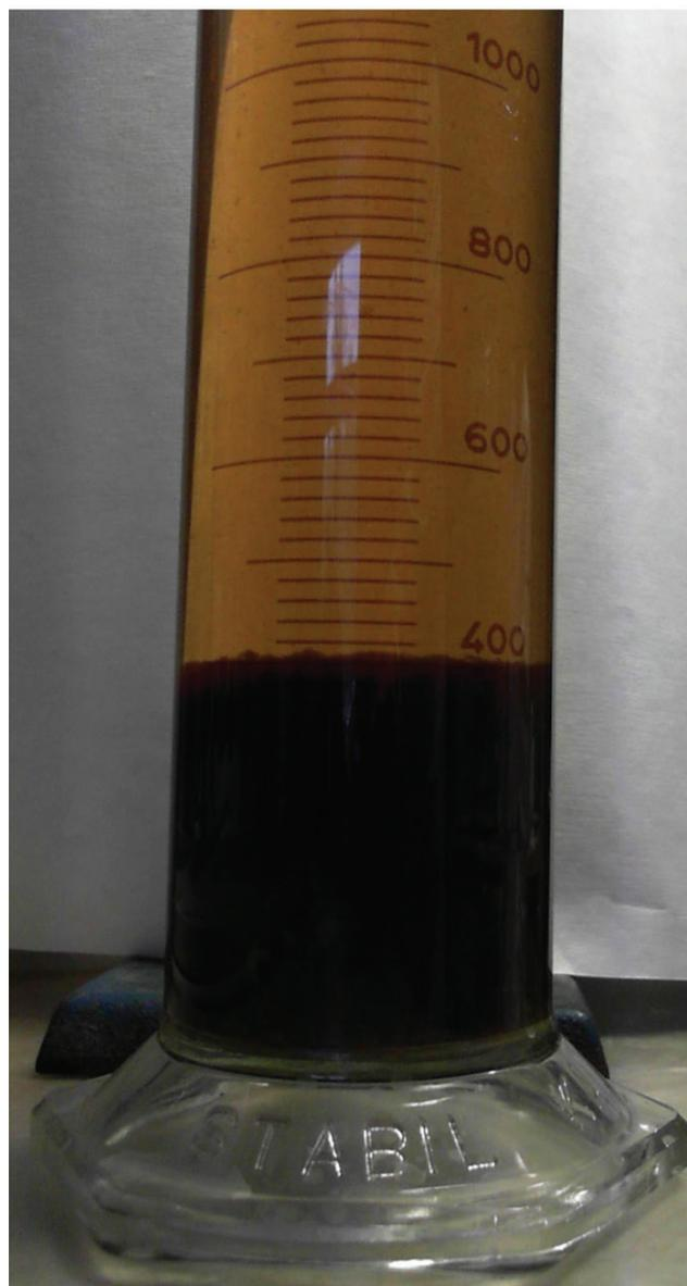
Fig. 3. Glycol after 24 h sedimentation. The glycol rubber was 20 vol% of cylinder after sedimentation.
