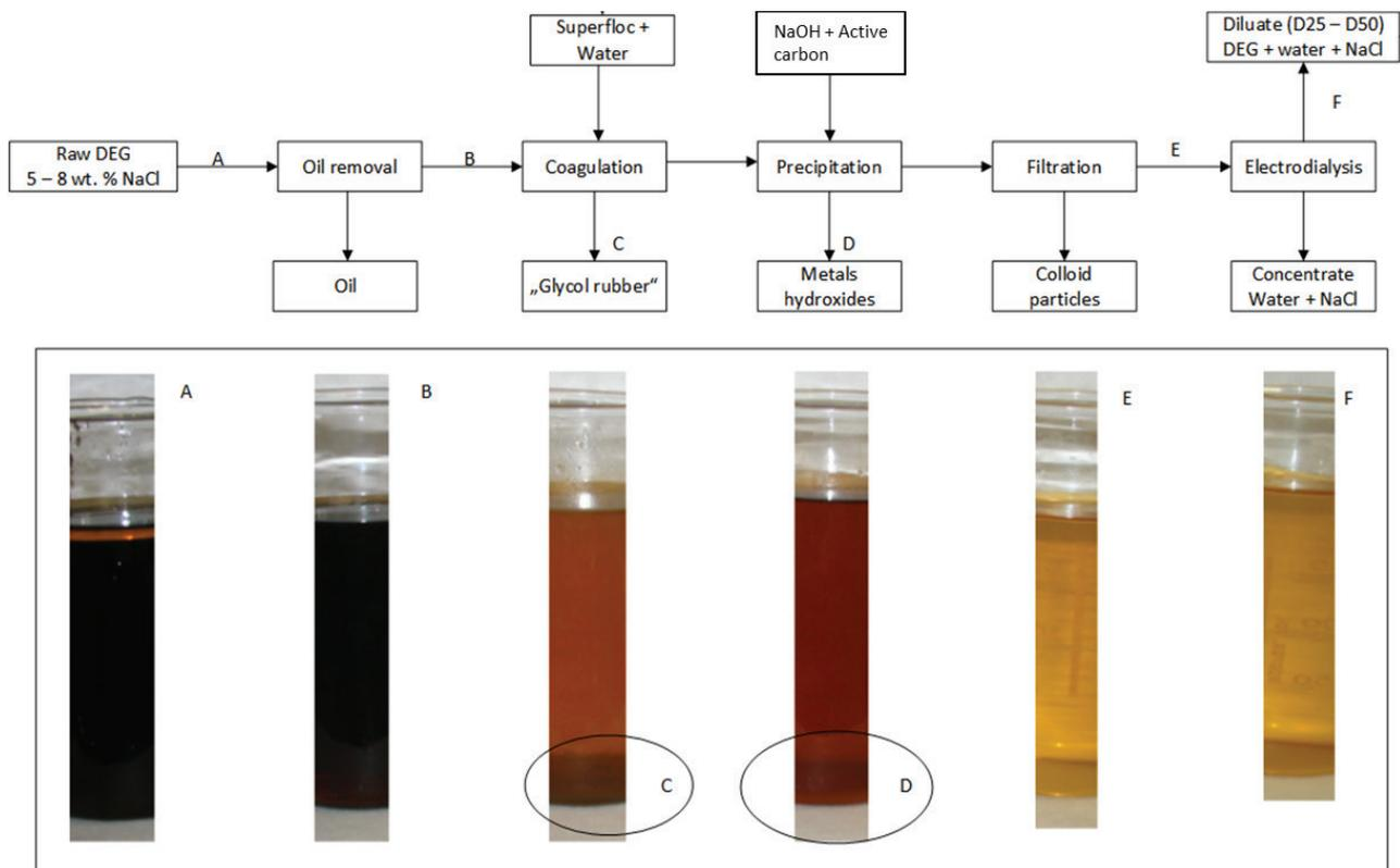
Fig. 9. PFD of the purification technology with products taken in each step.
