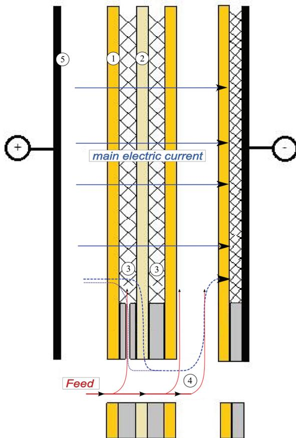
Fig. 3. Stack cross-section: pathway of shunt current in membrane and distributors area (standard electro dialysis stack). 1 – CM membrane, 2 – AM membrane, 3 – separator/manifold with oriented distributor, 4 – feeding channel and 5 – electrode.
