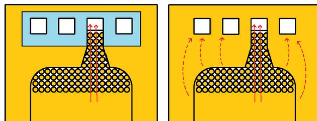
Fig. 1. Left: Illustration of shunt current path in innovated membrane with non-conductive inset (blue) and separator in order to electrically insulate the membrane active area from liquid distribution system (feeding channels). Right: Illustration of shunt current path in the standard membrane with separator.
