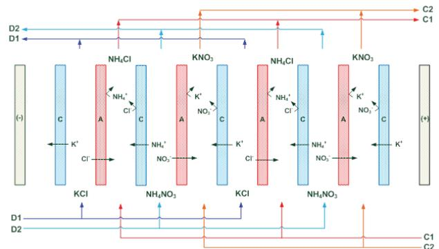
Fig. 4. Principle of potassium nitrate production by electro dialysis–metathesis.
