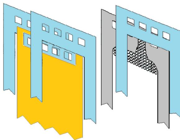
Fig. 2. Spacer (gray) with thin plastic cover (blue) on both sides in order to insulate feed and drain channels from ion-exchange membranes and membrane (yellow) by inset and thin plastic cover (blue) completely insulated from distribution system.
