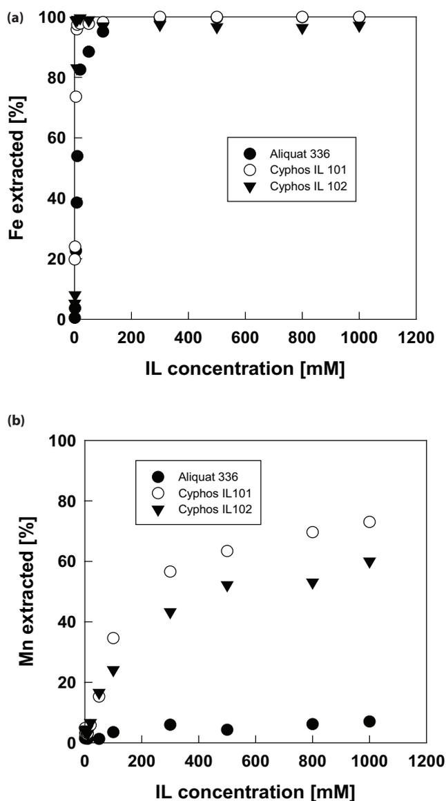
Fig. 3. Influence of ionic liquid concentration on the extractability of Fe(III) (a) and Mn(II) (b). Hydrochloric acid concentration is 4.0 M.
