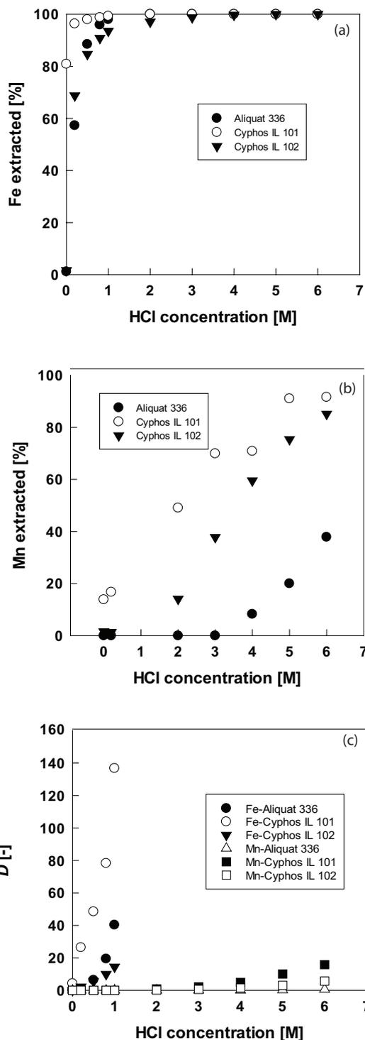
Fig. 2. Influence of HCl concentration on extractability of Fe(III) (a), Mn(II) (b), and the distribution ratio of Fe(III) and Mn(II) (c). Concentration of ionic liquid is 1.0 M.
