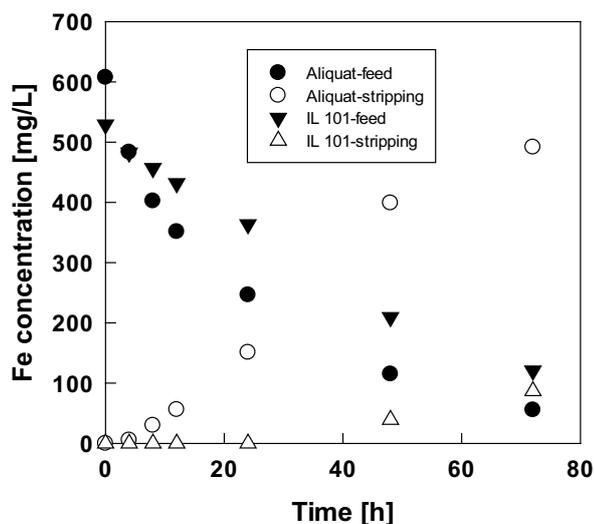
Fig. 4. Permeation of Fe(III) using Aliquat 336 and Cyphos IL 101 as carrier.
