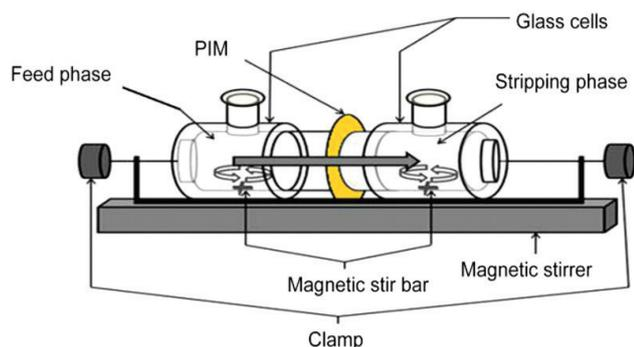
Fig. 1. Schematic diagram of the experimental setup for the permeation experiment.
