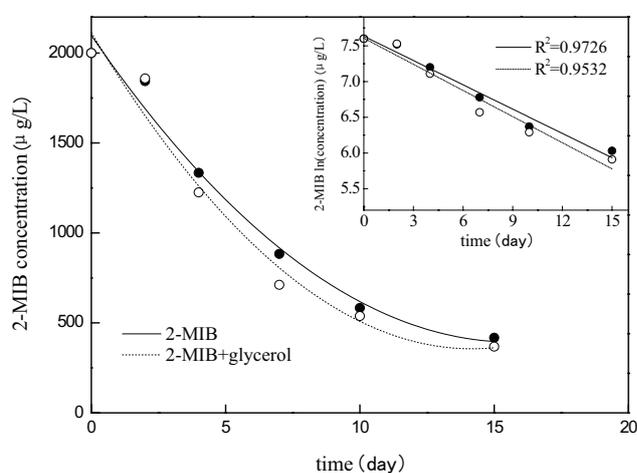
Fig. 12. Kinetics of 2 mg/L 2-MIB biodegradation for *B. idriensis*.
