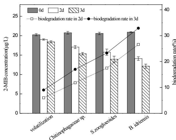
Fig. 4. Degradation efficiency of 2-MIB by three strains.
