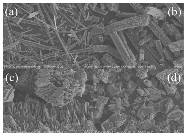
Fig. 12. SEM images of calcium sulfate crystals: in the absence of AA-TPEL (a) and in the presence of AA-TPEL: (b) 1 mg L<sup>-1</sup>, (c) 2 mg L<sup>-1</sup> and (d) 3 mg L<sup>-1</sup>.
