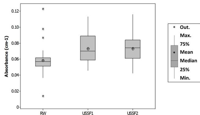
Fig. 8. Boxplot of 254 nm absorbance of raw and filtered water ( $n = 42$ ).
