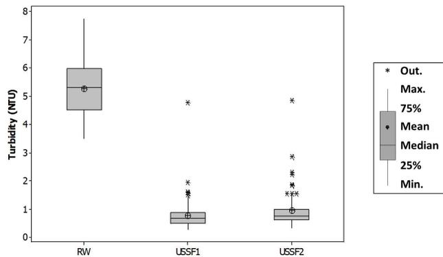
Fig. 2. Boxplot of turbidity data of raw and filtered water ( $n = 81$ ).
