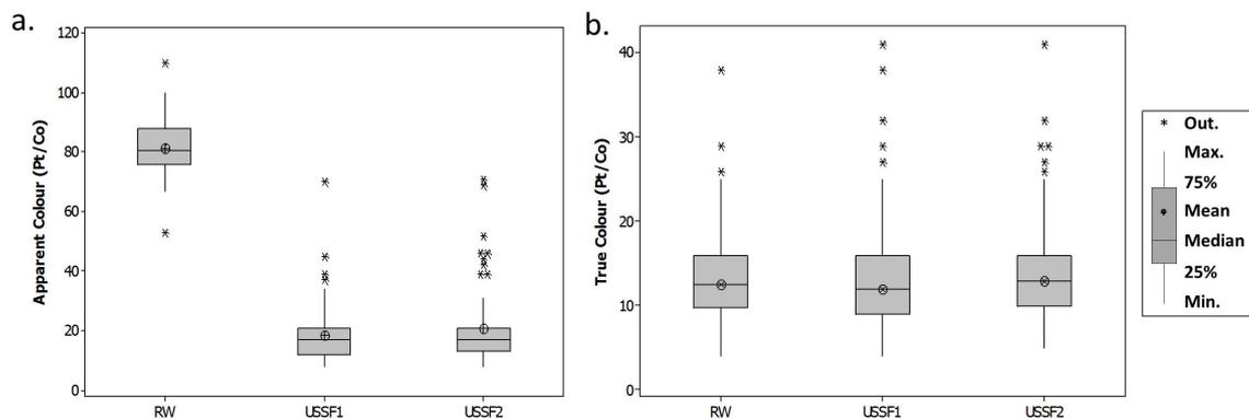
Fig. 3. Boxplot of apparent (a) and true (b) colour data of raw and filtered water ( $n = 81$ ).
