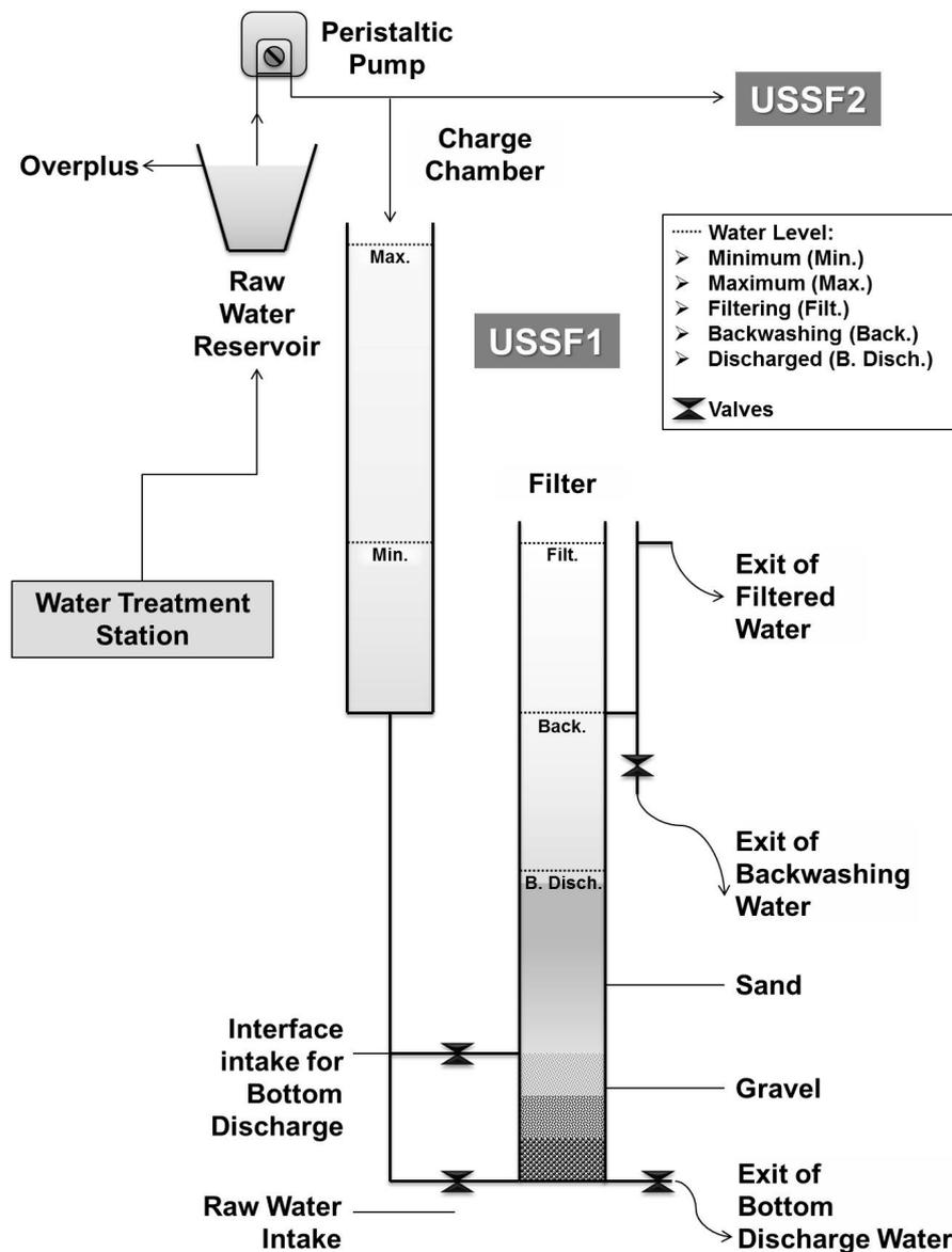
Fig. 1. The upflow slow sand filter system.
