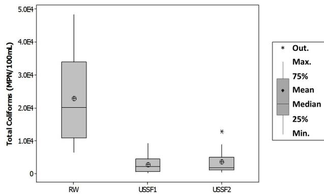
Fig. 4. Boxplot of total coliform data of raw and filtered water ( $n = 12$ ).
