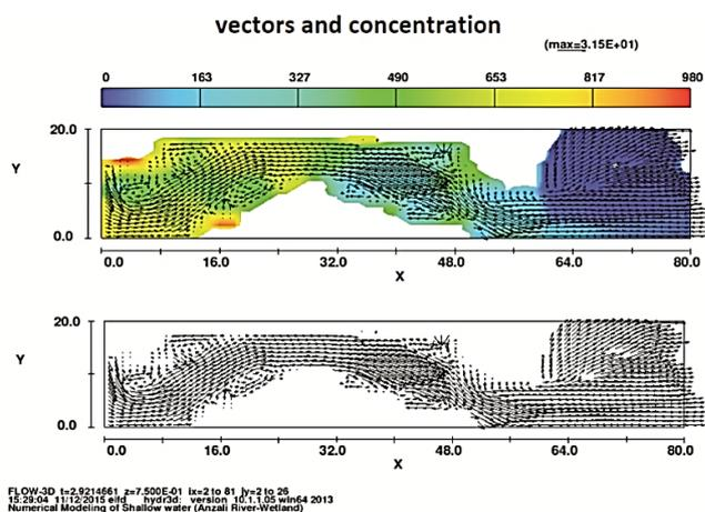
Fig. 11. Distribution of the element of horizontal velocity and direction along the waterway using the simulator.
