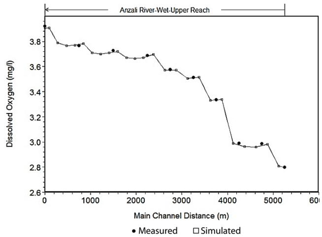
Fig. 9. Comparison between the annual changes of the calculated and measured DO.
