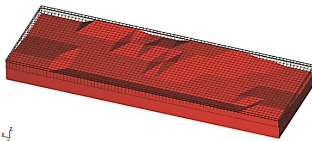
Fig. 3. Computational field, number of elements, and geometry of the study region.
