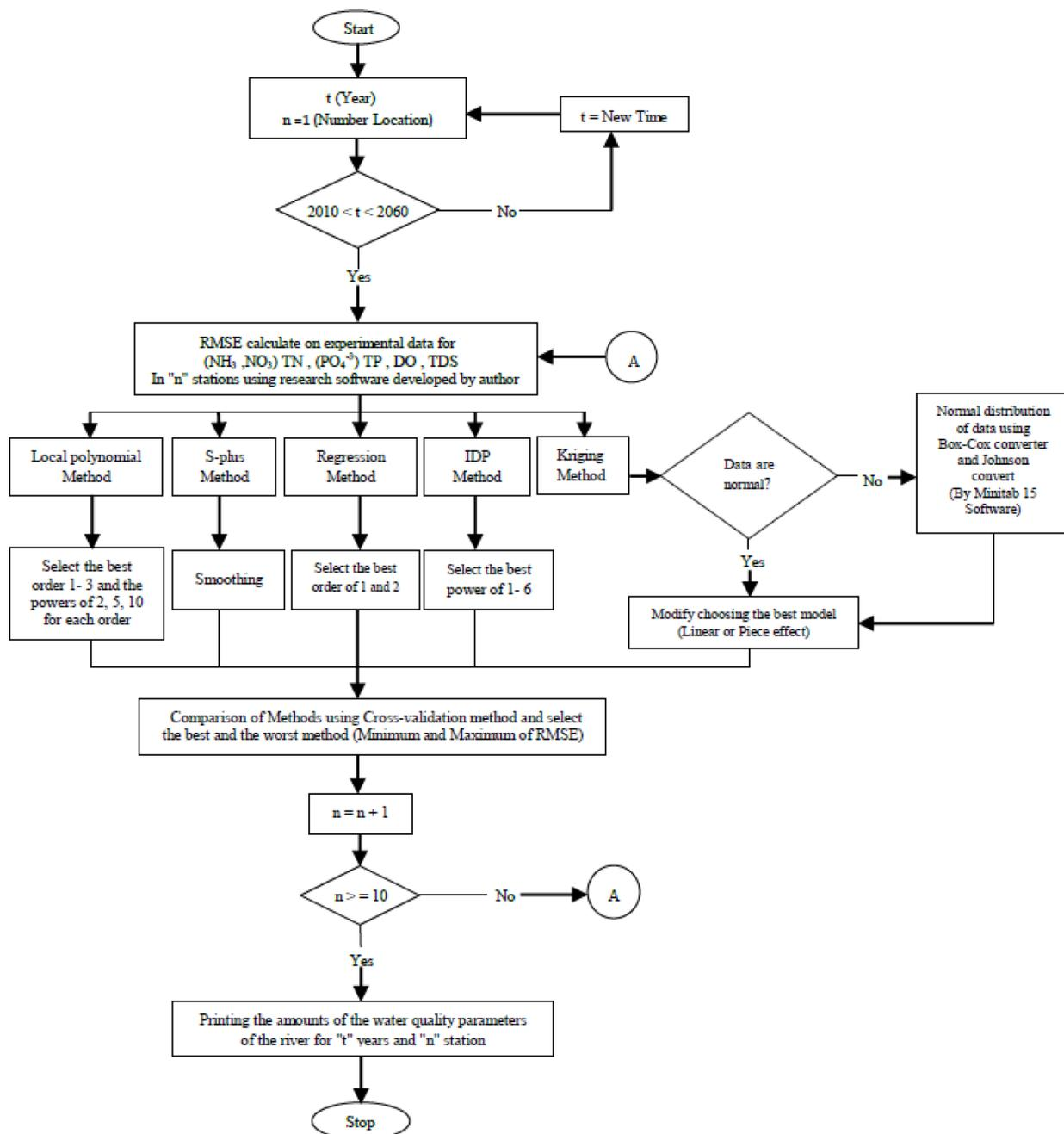
Fig. 4. Flowchart of water quality model for estimating the nutrient.
