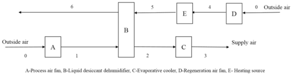
Fig. 1. Simplified flow diagram of liquid desiccant cooling system.
