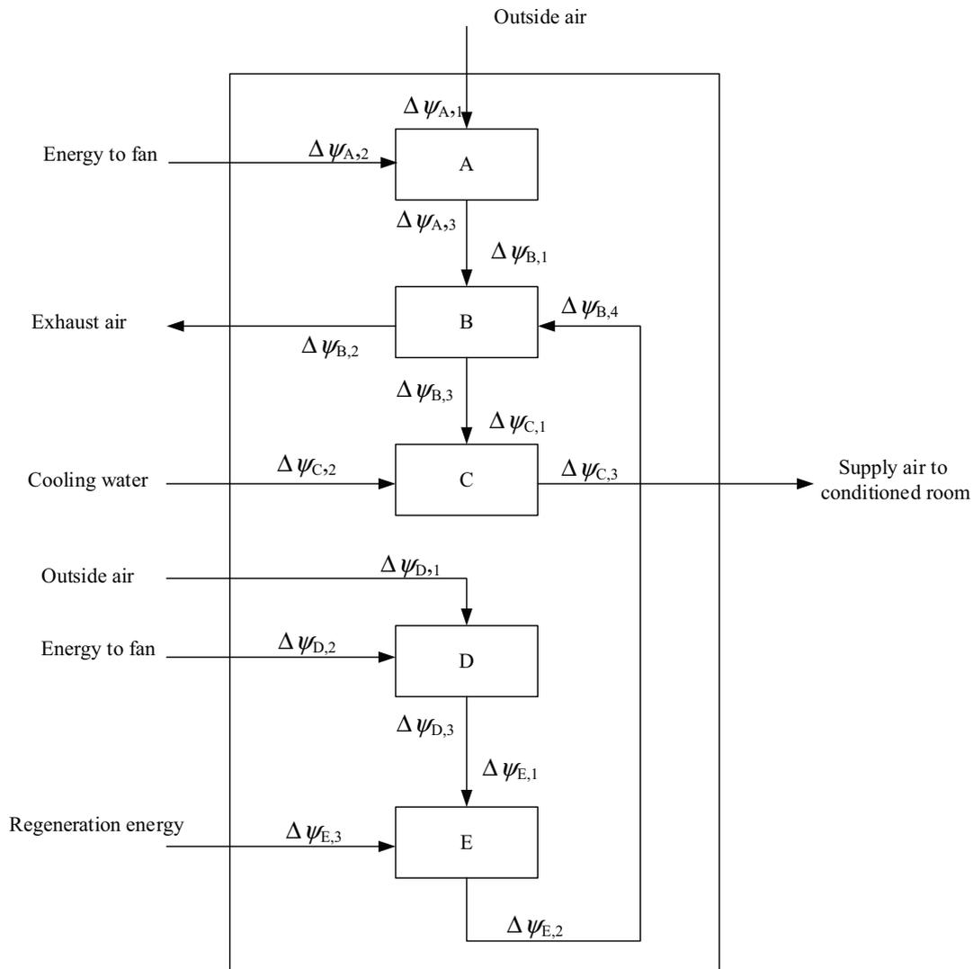
Fig. 2. Thermo-economic functional diagram of liquid desiccant cooling system.
