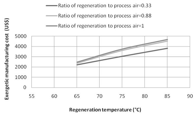
Fig. 6. Variations of exergetic manufacturing cost with regeneration temperature and ratio of mass flow rates.
