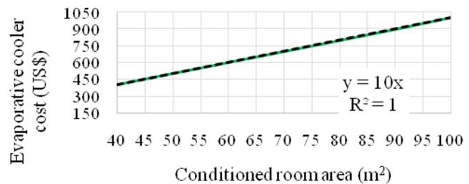
Fig. 5. Cost of evaporative cooler.
