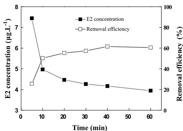
Fig. 1. E2 concentration in solution and E2 removal efficiency at different time.
