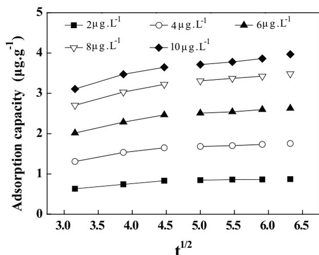
Fig. 9. Intraparticle diffusion plots for the adsorption of E2 by AnGS.
