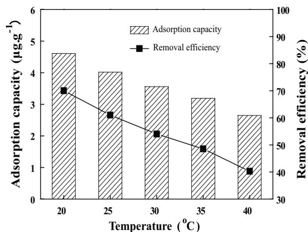
Fig. 4. Effect of temperature on E2 adsorption by AnGS.
