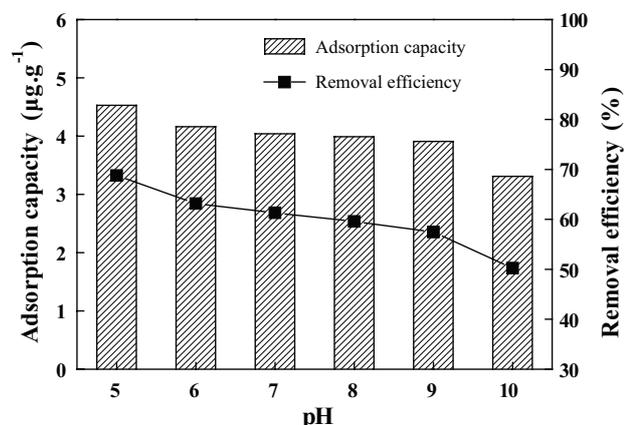
Fig. 5. Effect of pH on E2 adsorption by AnGS.
