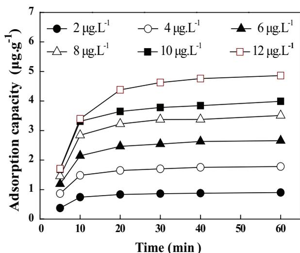
Fig. 2. Effect of initial E2 concentration on E2 adsorption by AnGS.
