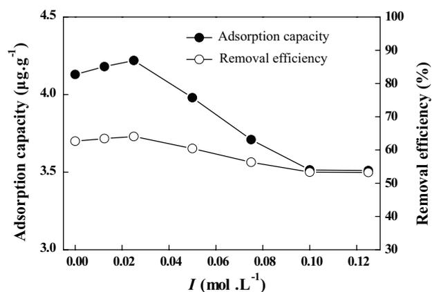
Fig. 6. Effect of ionic strength (NaCl) on E2 adsorption by AnGS.
