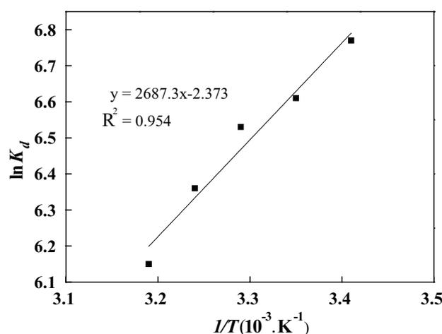
Fig. 8. Thermodynamic plot for the adsorption of E2 by AnGS.
