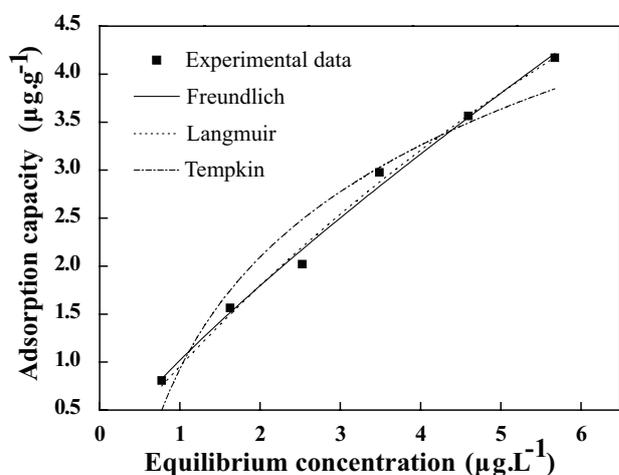
Fig. 7. Isotherm plots for the adsorption of E2 by AnGS.
