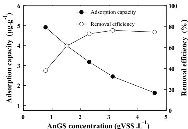
Fig. 3. Effect of AnGS concentration on E2 adsorption by AnGS.
