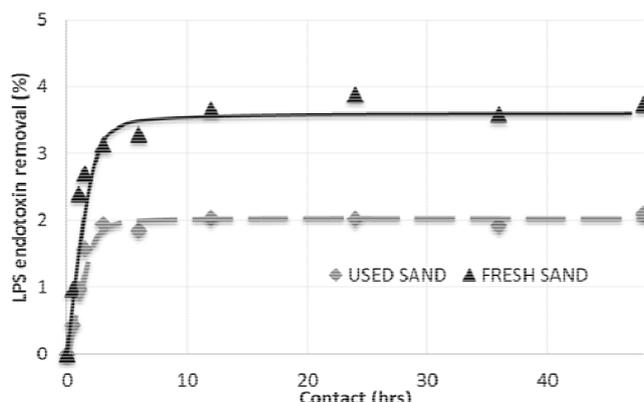
Fig. 6. LPS endotoxin adsorption: used sand vs. fresh sand.
