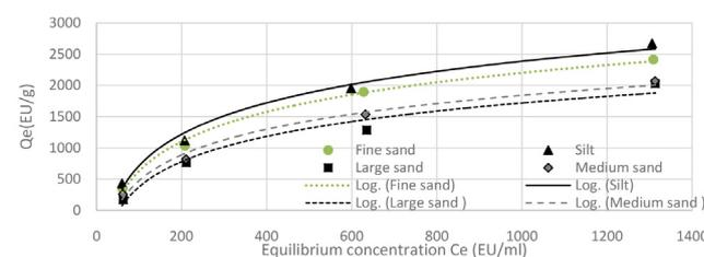
Fig. 7. LPS endotoxin adsorption amount per mass unit of soil versus equilibrium concentration.
