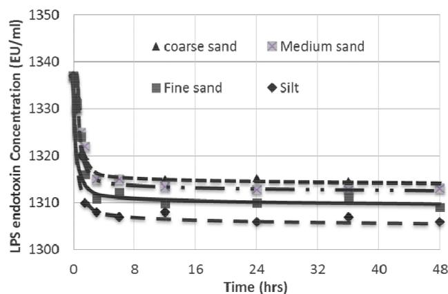
Fig. 4. Effect of the contact time on the LPS endotoxin adsorption into soil.
