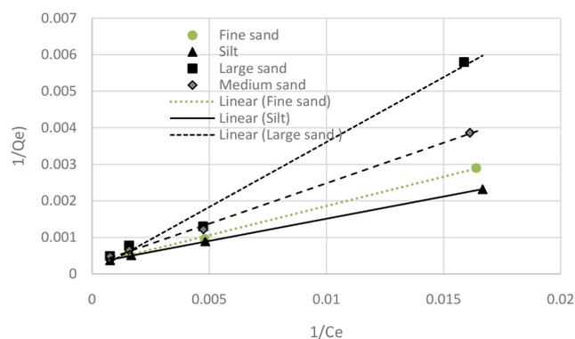
Fig. 9. Langmuir adsorption isotherm for LPS endotoxin.
