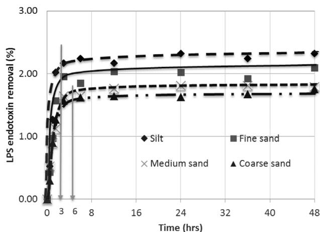
Fig. 1. Effect of soil type on the LPS endotoxin removal efficiency (soil dose 5.8 g/L).
