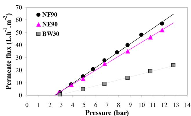
Fig. 2. Permeate flux dependence on applied pressure for the tested membranes (pH = 7.9, T = 21°C, Feed TDS 4 g·L<sup>-1</sup>).
