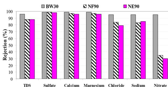
Fig. 3. Average Rejection of TDS and common ions in feed water by the investigated membranes (Y = 70%, permeate flux = 26 L·m<sup>-2</sup>·h<sup>-1</sup>, T = 21°C).
