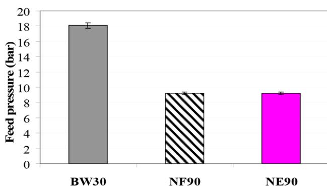
Fig. 4. Feed pressures required for Tan Tan water desalination by the investigated membranes ( $Y = 70\%$ , permeate flux = 26 L·m<sup>-2</sup>·h<sup>-1</sup>,  $T = 21^\circ\text{C}$ ).
