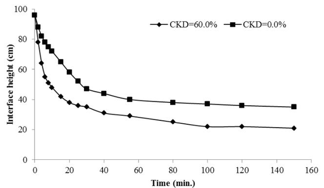
Fig. 2. Relation between sludge interface height and settling time.
