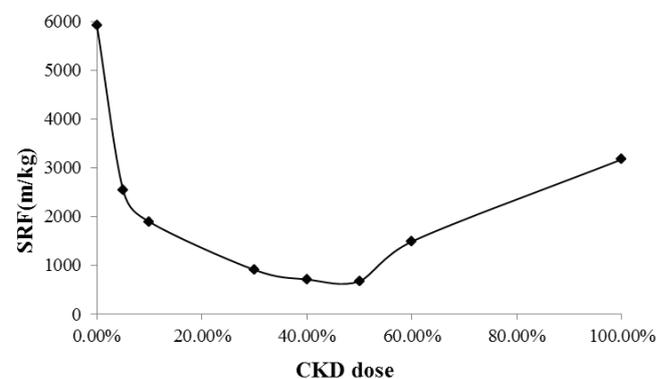
Fig. 4. Relation between specific resistance of filtration and CKD dosage.
