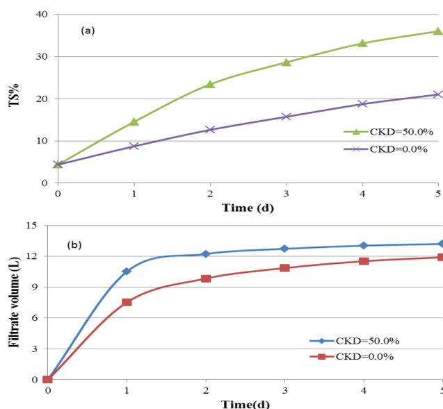
Fig. 5. Relation between drying time and (a) sludge solid content and (b) filtrate volume.
