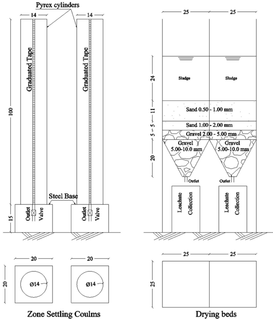
Fig. 1. Zone settling columns and drying beds pilot.
