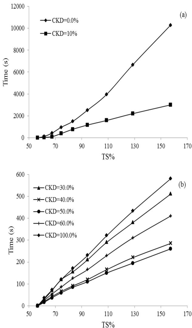
Fig. 3. Relation between sludge solid content and filtrate time for different CKD dosage.
