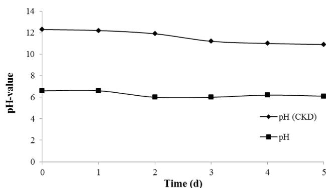
Fig. 6. Relation between drying time and pH value for treated and untreated sludge.
