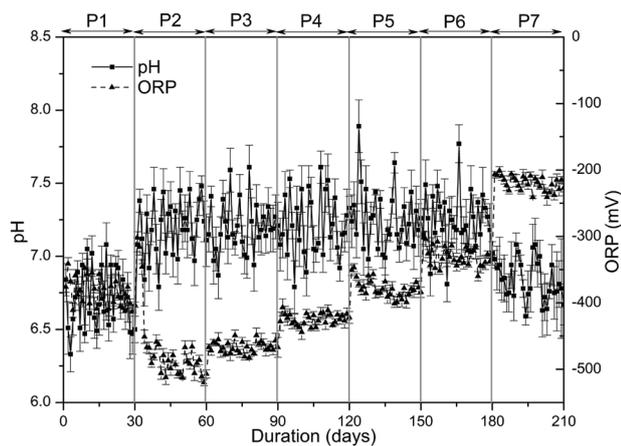
Fig. 4. Variation of pH (■) and ORP (▲) under anaerobic and microaerobic conditions during semi-continuous digestion of activated sludge supplemented with RSI.
