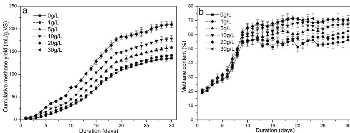
Fig. 1. Effect of RSI dosages on  $\text{CH}_4$  production during batch digestion of activated sludge: (a)  $\text{CH}_4$  yield and (b)  $\text{CH}_4$  content.
