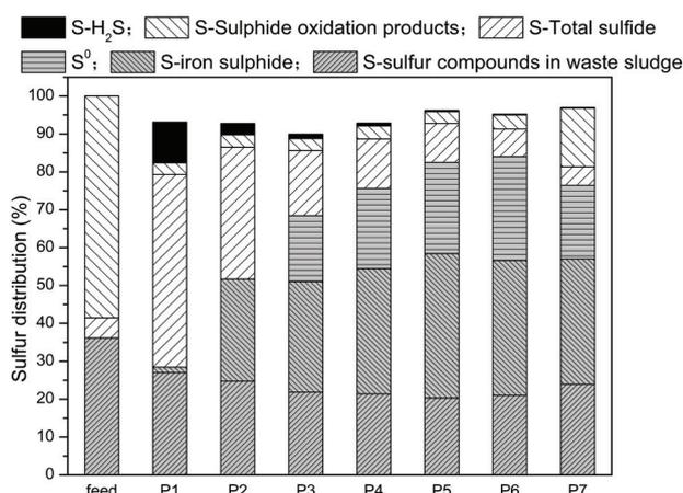
Fig. 7. Calculated sulfur balance during semi-continuous anaerobic and microaerobic digestion of activated sludge supplemented with rusty scrap iron (RSI) over seven periods of operation associated with stepwise increases in oxygen concentration: (1) sulfur compounds in waste sludge, (2) iron sulfide precipitation, (3) elemental sulfur  $\text{S}^0$ , (4) sulfide in liquid phase, (5) sulfide oxidation products and (6) sulfur in biogas.
