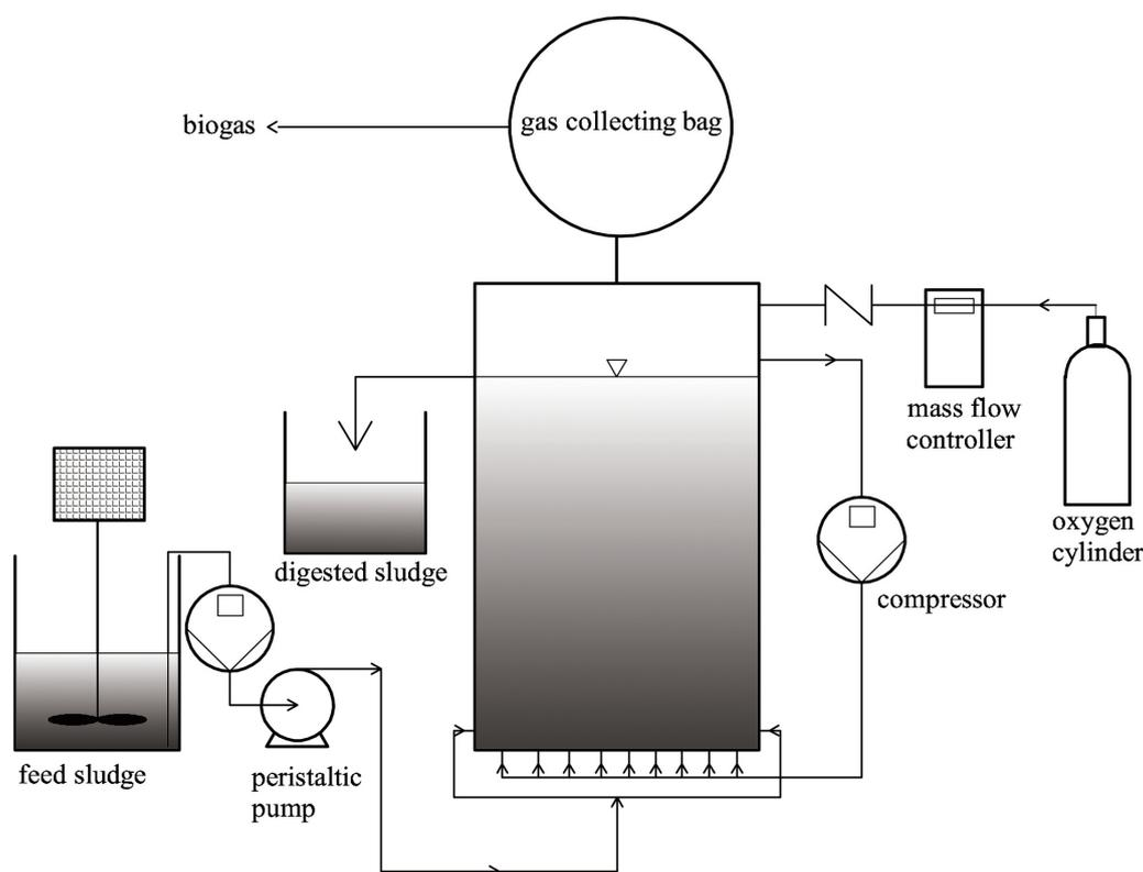
Fig. S1. Lab-scale bioreactor diagram for semi-continuous anaerobic and microaerobic digestion of activated sludge supplemented with rusty scrap iron (RSI).
