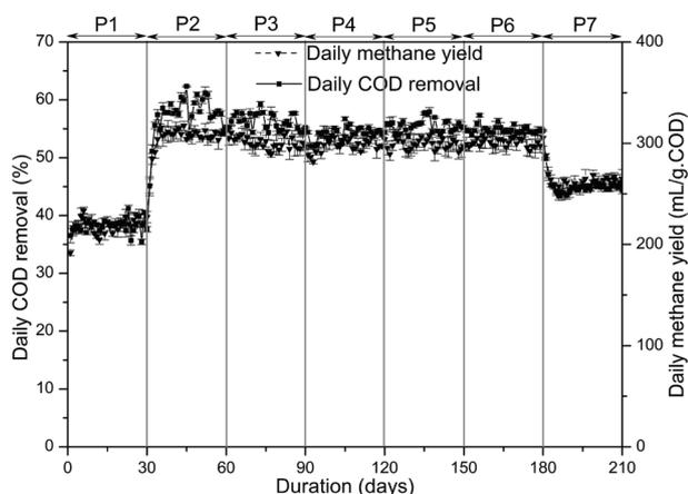
Fig. 5. Daily COD removal (■) and daily methane yield (▼) under anaerobic and microaerobic conditions during the digestion of sludge.
