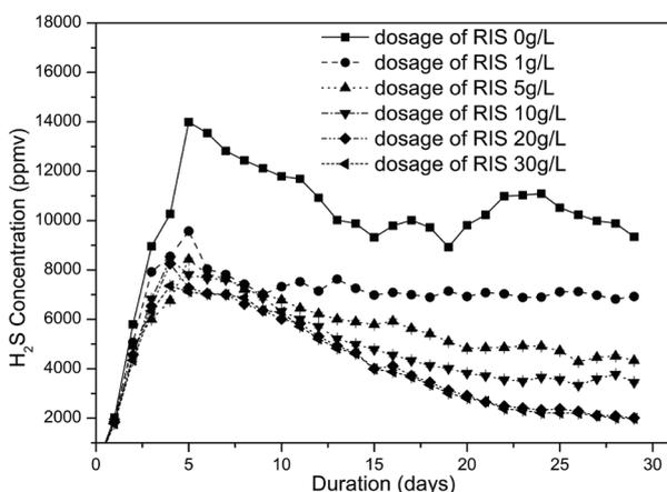
Fig. 3. H<sub>2</sub>S concentrations present in biogas from batch digestion of activated sludge in the presence of different RSI dosages (error bars represent standard deviation,  $n = 3$ ).
