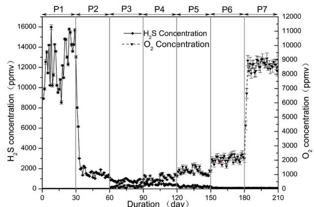
Fig. 6. Hydrogen sulfide (◆) and oxygen (▼) concentrations under anaerobic and microaerobic conditions during semi-continuous digestion of activated sludge supplemented with RSI.
