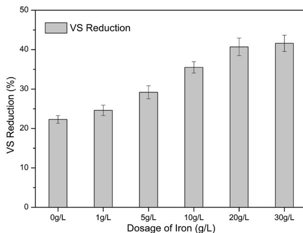
Fig. 2. Effect of RSI dosages on VS reduction during batch digestion of activated sludge.
