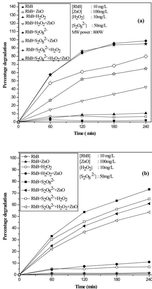
Fig. 8. Degradation of RhB using different combination of additives. (A) Under MW irradiation and (B) under conventional heating.
