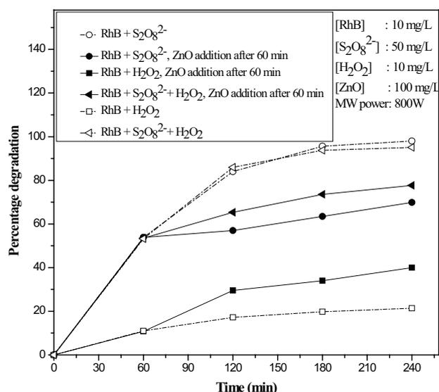
Fig. 10. Effect of in-between addition of ZnO on MW degradation of RhB.
