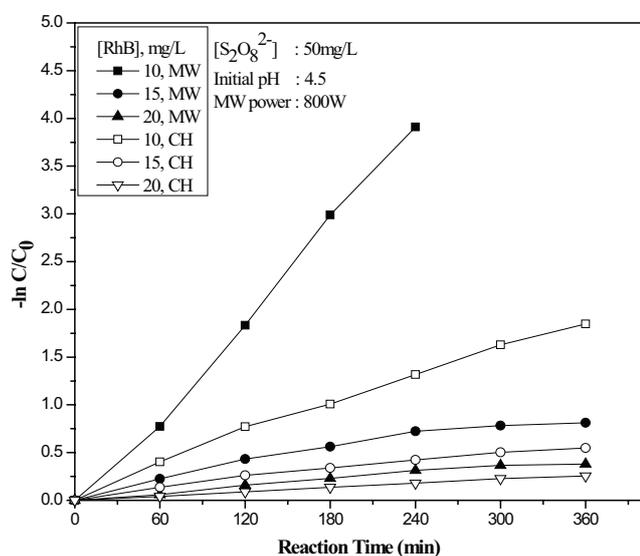
Fig. 4. Logarithmic plot for the degradation of RhB under MW irradiation and conventional heating (CH).
