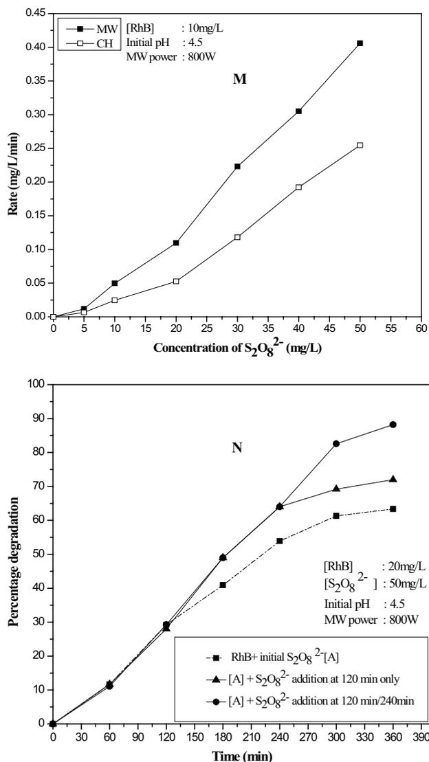
Fig. 3. (M) Effect of concentration of  $S_2O_8^{2-}$  on the rate of degradation of RhB. (N) Effect of in-between addition of  $S_2O_8^{2-}$  on MW degradation of RhB.
