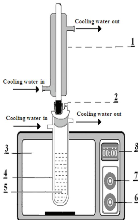
Fig. 1. Schematic representation of the reactor assembly; (1) condenser, (2) thermometer pocket/sampling port, (3) microwave oven cavity, (4) reactor, (5) reaction solution/suspension, (6) power adjuster, (7) timer and (8) time display.
