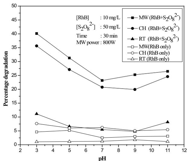
Fig. 7. Effect of pH on the degradation of RhB.
