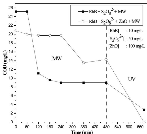
Fig. 11. Variation of COD with time during the MW/S<sub>2</sub>O<sub>8</sub><sup>2-</sup> degradation of RhB: effect of ZnO and UV irradiation.
