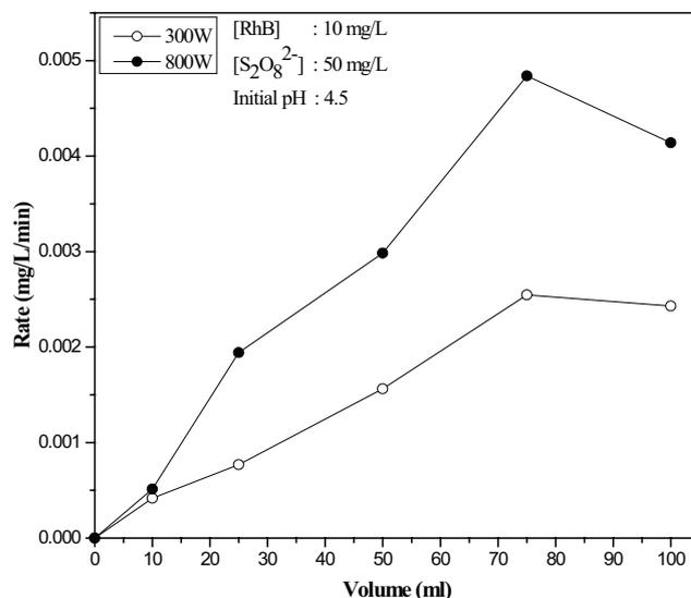
Fig. 6. Effect of MW power on rate of RhB degradation at different volumes.
