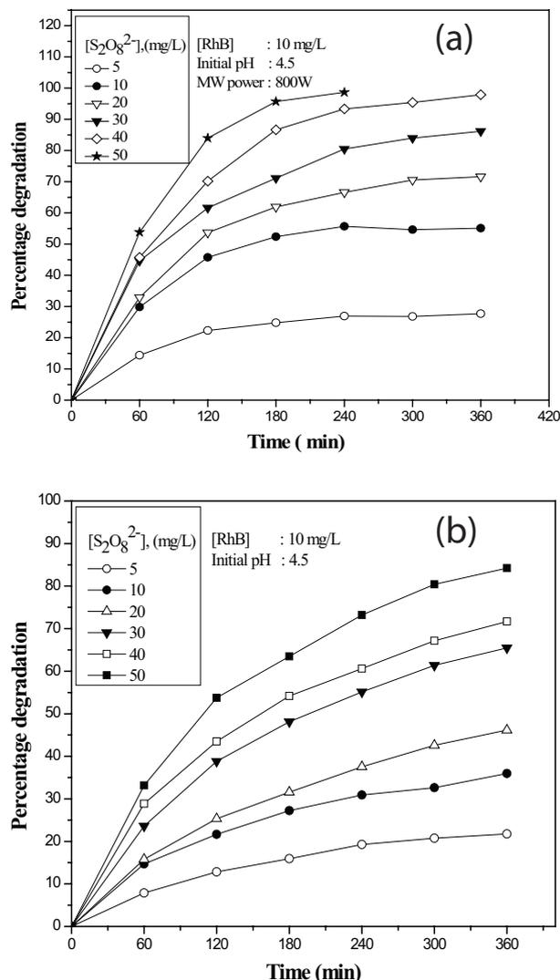
Fig. 2. Effect of  $S_2O_8^{2-}$  concentration on the degradation of RhB. (A) Under MW irradiation and (B) under conventional heating.
