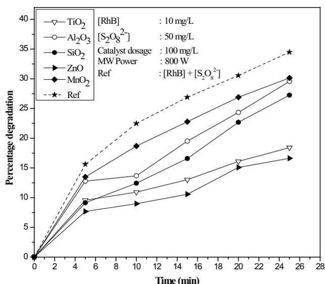
Fig. 9. Effect of different suspended oxides on MW/ $S_2O_8^{2-}$  degradation of RhB.
