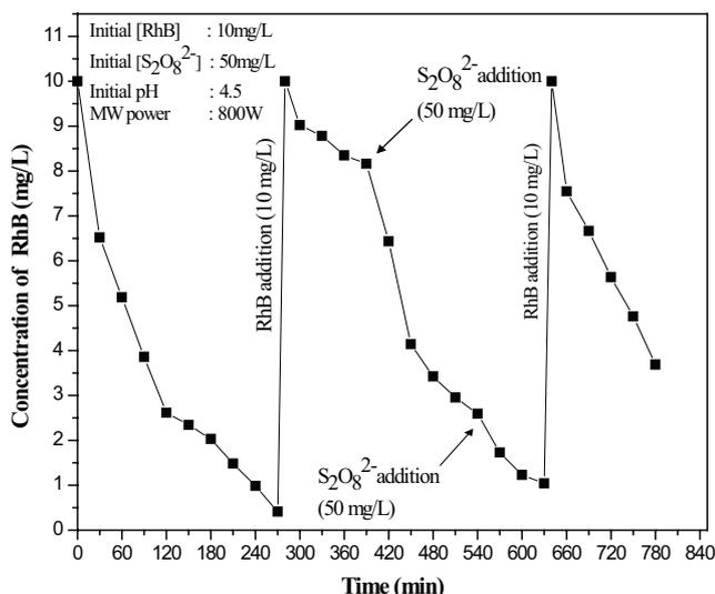
Fig. 5. Effect of in-between addition of RhB/ $\text{S}_2\text{O}_8^{2-}$  on MW degradation of RhB.
