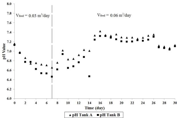
Fig. 7. pH values throughout the 30-d feeding process of pilot-scale ABD (second operation).
