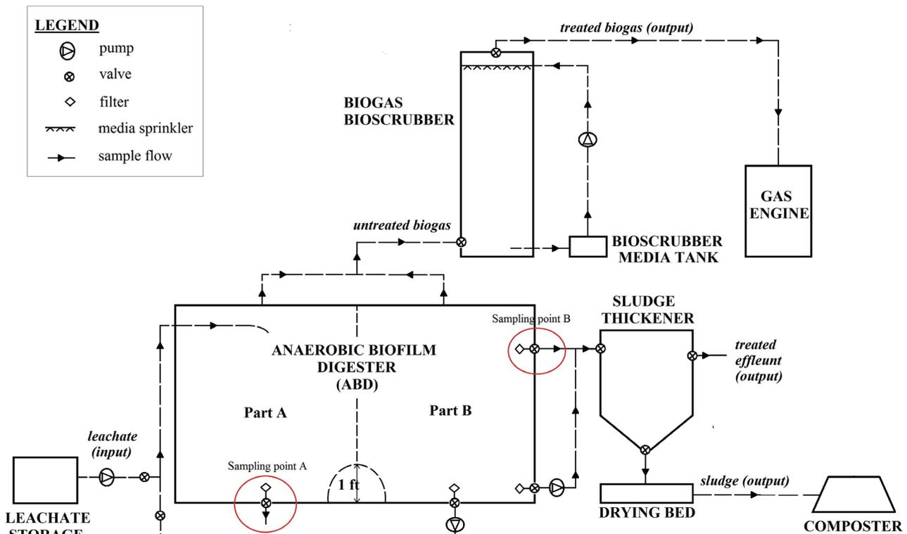
Fig. 1. Schematic drawing of a complete pilot-scale ABD system.
