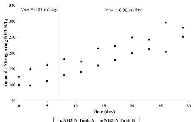
Fig. 11. NH<sub>3</sub>-N values throughout the 30-d feeding process of pilot-scale ABD (second operation).
