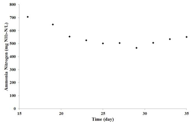
Fig. 6.  $\text{NH}_3\text{-N}$  values from day 16 to day 35 in the pilot-scale ABD (first operation).
