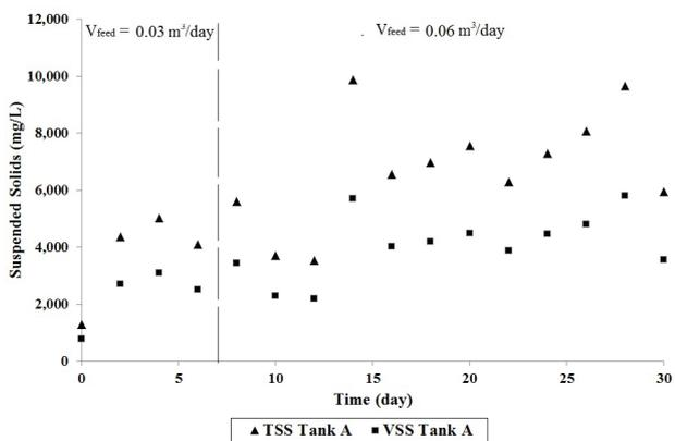
Fig. 8. TSS and VSS values for Tank A during feeding process of pilot-scale ABD (second operation).
