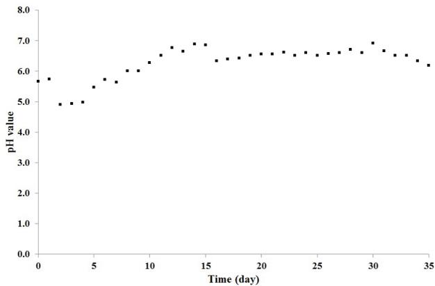
Fig. 3. pH values throughout the feeding process of pilot-scale ABD (first operation).
