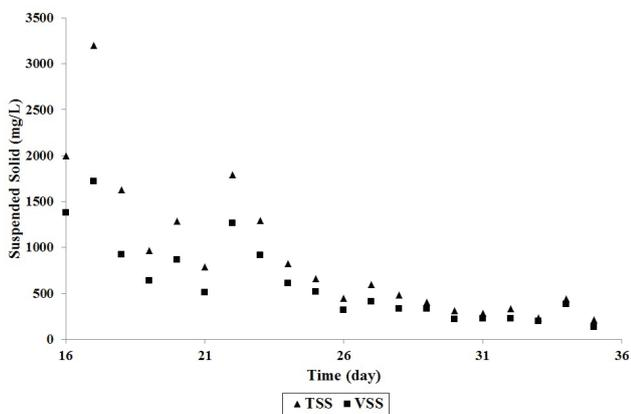
Fig. 4. TSS and VSS values from day 16 to day 35 during feeding process of pilot-scale ABD (first operation).
