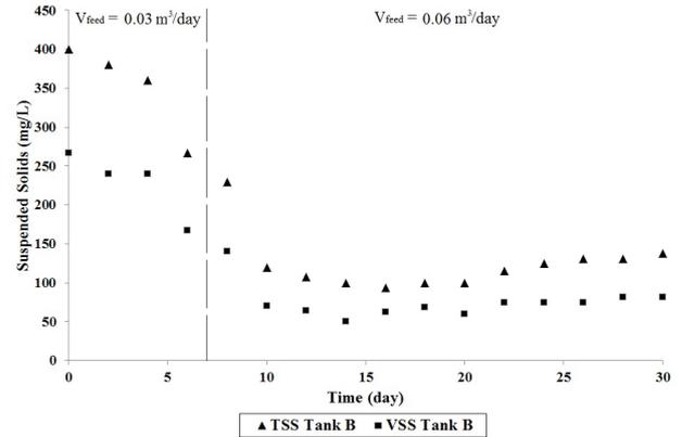
Fig. 9. TSS and VSS values for Tank B during feeding process of pilot-scale ABD (second operation).
