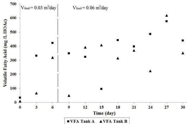
Fig. 12. Total VFA values throughout the 30-d feeding process of pilot-scale ABD (second operation).
