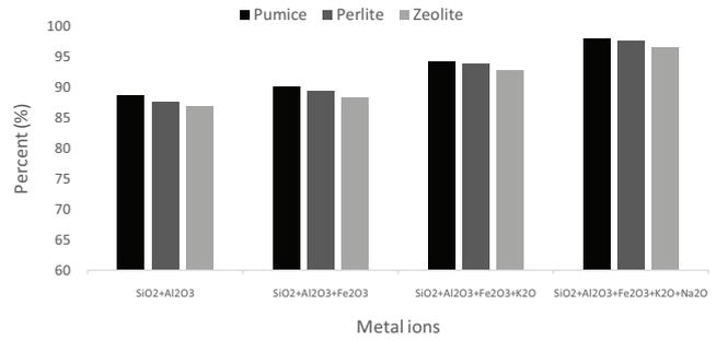
Fig. 8. Presence of metal ions in raw aggregates.
