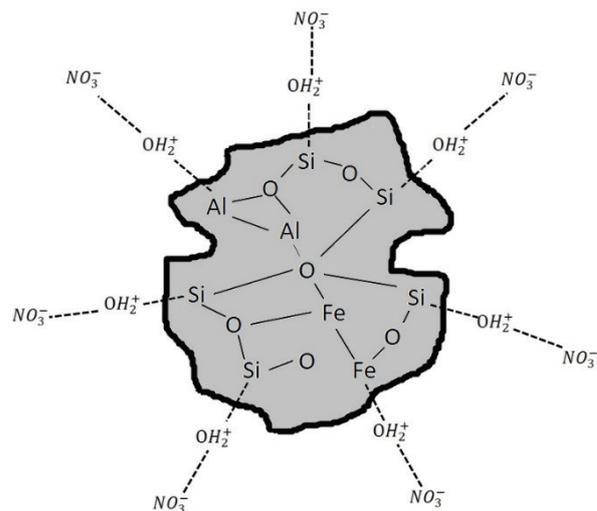
Fig. 10. Mechanism of nitrate absorption using metal ions in aggregates.
