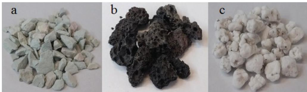
Fig. 1. The aggregates used in this research (a) zeolite, (b) pumice, and (c) perlite.
