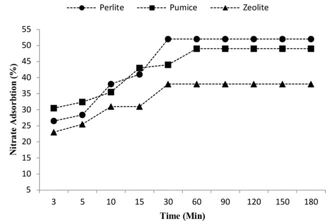
Fig. 6. Nitrate adsorption by H<sub>2</sub>SO<sub>4</sub> activated aggregates.
