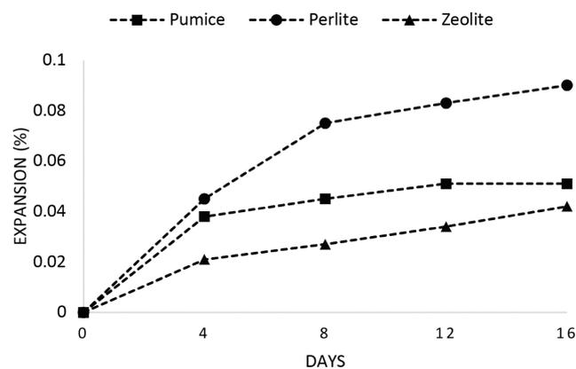
Fig. 3. Results of alkali-silica reaction test (expansion of specimens).
