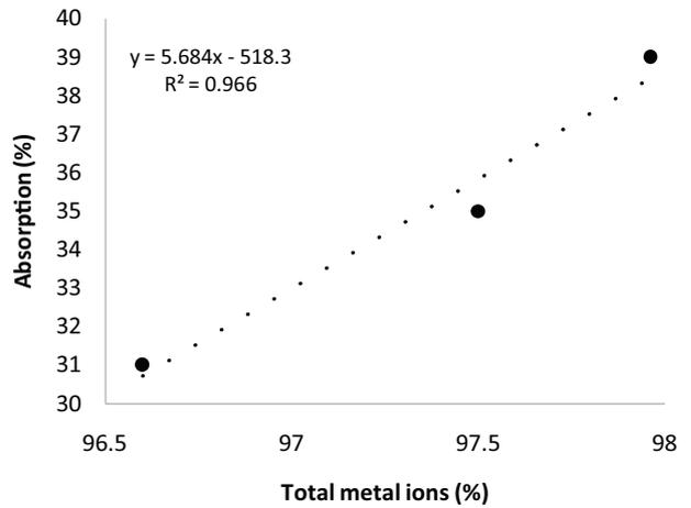
Fig. 9. Relation between absorption and total metal ions in raw aggregates.
