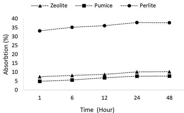
Fig. 2. Water absorption of aggregates at different times.
