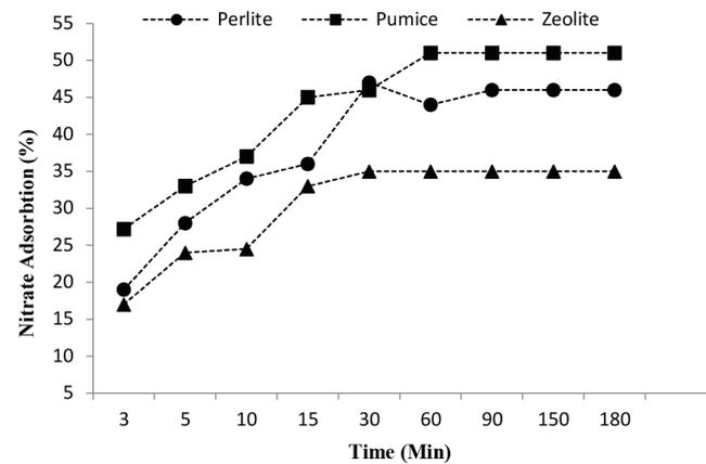
Fig. 5. Nitrate adsorption by HCl activated aggregates.
