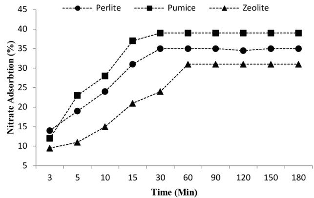
Fig. 4. Nitrate adsorption by raw aggregates.
