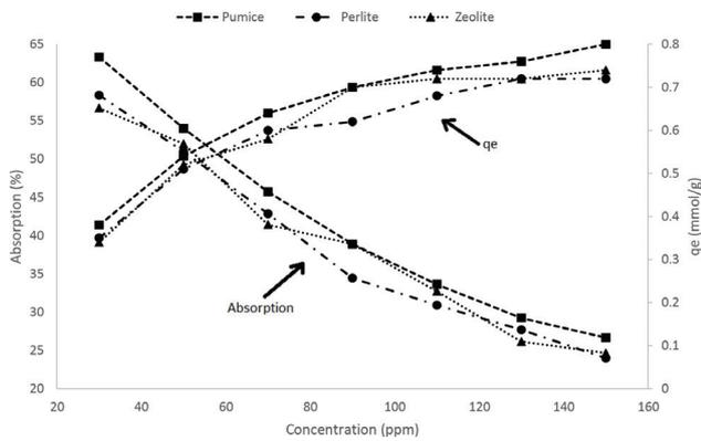
Fig. 7. Nitrate absorption and adsorbent capacity of aggregates vs. nitrate concentration.
