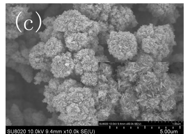
Fig. 6. SEM images of PPy-SDBS/Ti electrode (a), Gr/PPy-SDBS/Ti electrode (b) and Pd/Gr/PPy-SDBS/Ti electrode (c).
