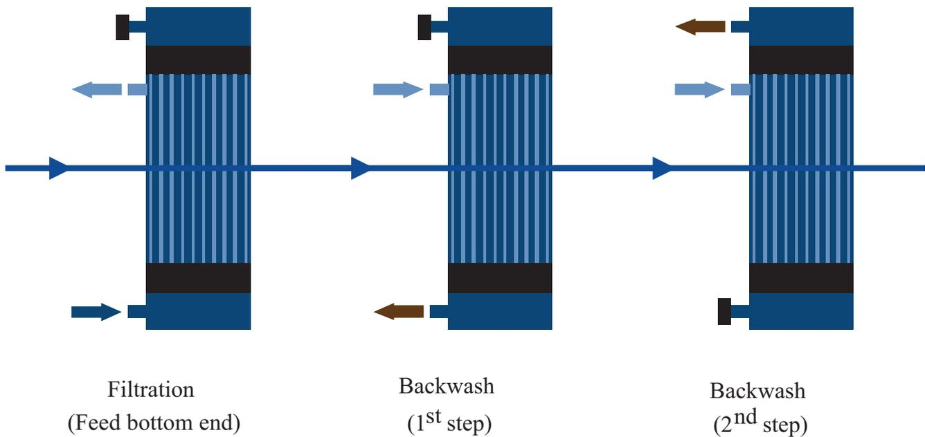
Fig. 3. Direction of flow in a Dizzer® module during filtration and backwash mode.
