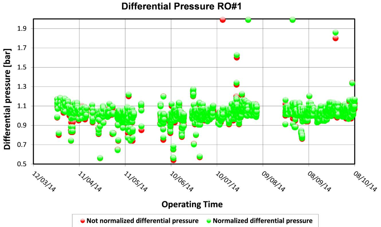
Fig. 6. Differential pressure in RO#1 pretreated by UF.
