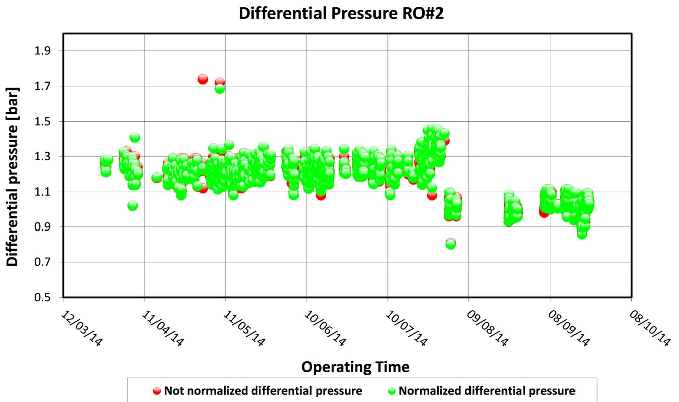
Fig. 7. Differential pressure in RO#2 pretreated by GMF.
