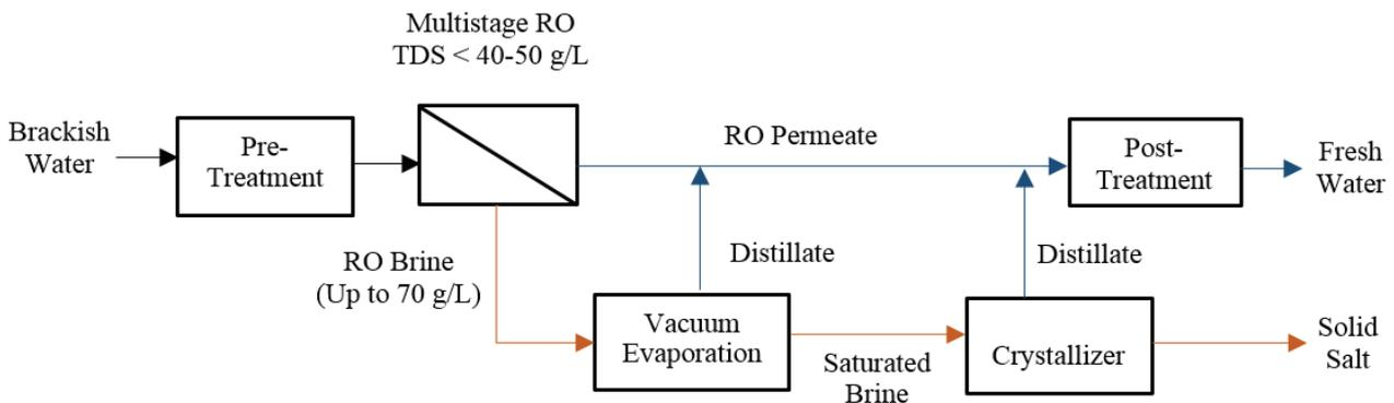
Fig. 4. Traditional ZLD 'lay-out' (municipal desalination).
