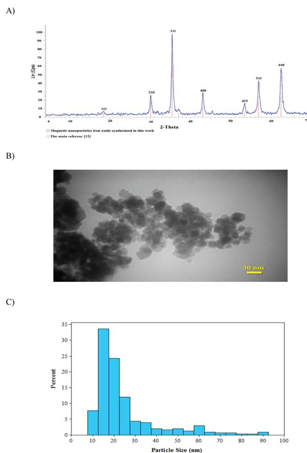
Fig. 3. (A) XRD pattern of synthesized Fe<sub>3</sub>O<sub>4</sub> NPs. (B) TEM image of synthesized Fe<sub>3</sub>O<sub>4</sub> NPs. (C) Size distribution of synthesized Fe<sub>3</sub>O<sub>4</sub> nanoparticles.
