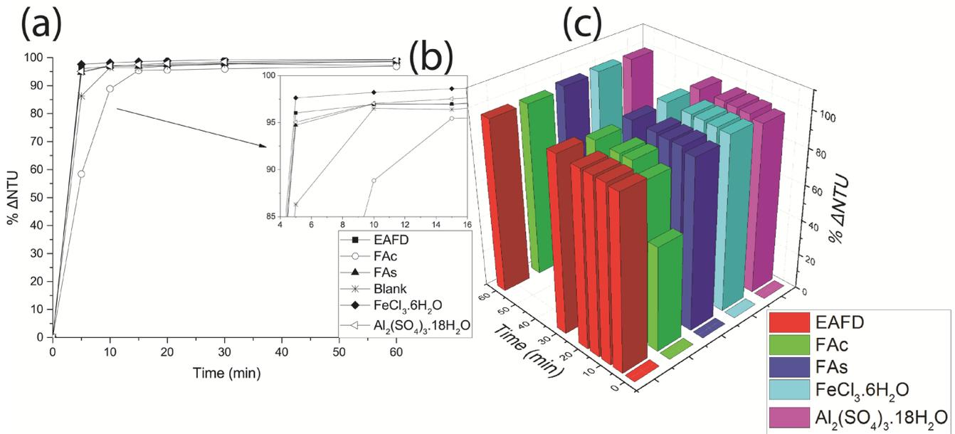
Fig. 4. The turbidity removal efficiency (% $\Delta$ NTU) as a function of time (min) for all coagulants tested in this study, at the optimal coagulant dosage (4 mg/L). Three different graphical representations are presented: (a) normal line and dot chart, (b) magnified inset of the upper-left (line overlapping) region as observed in the normal line and dot chart and (c) bar chart.
