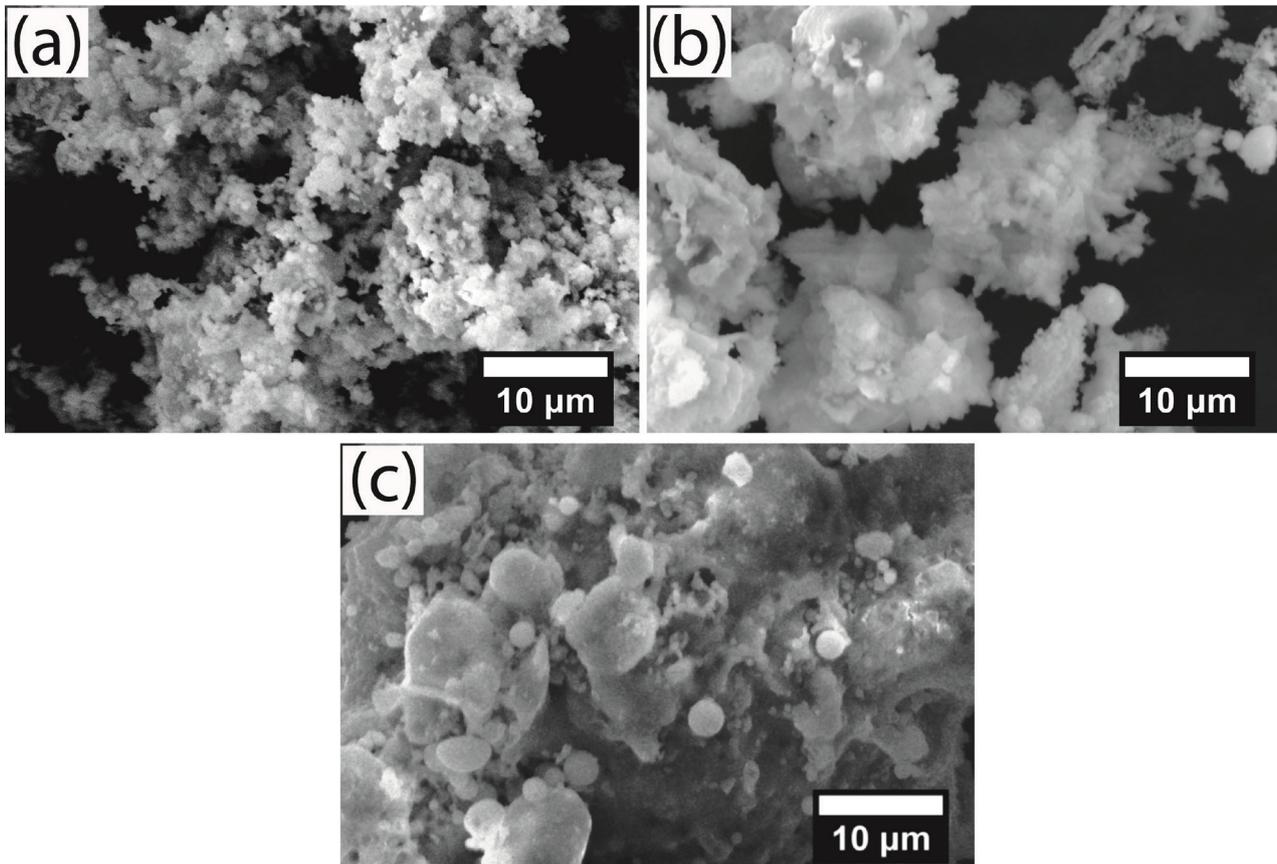
Fig. 1. SEM micrographs of the alternative coagulants used in this study: (a) EAFD, (b) FAc and (c) FAs.
