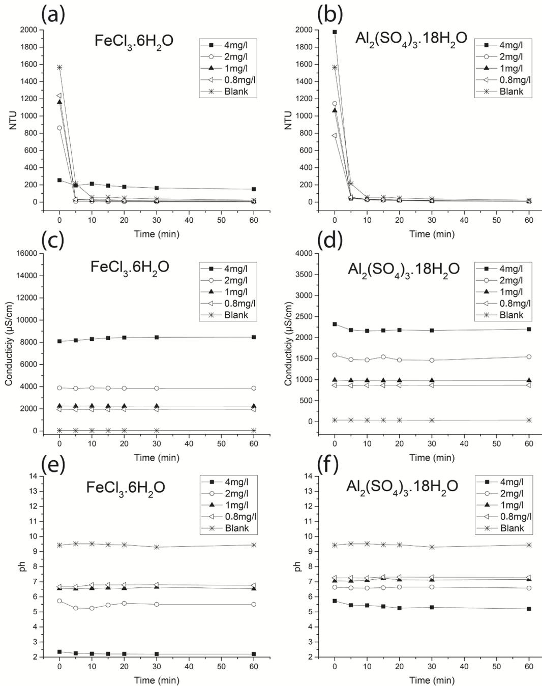
Fig. 3. Wastewater turbidity, NTU (a) and (b); electrical conductivity (c) and (d); and pH (e) and (f) as a function of time (min), using two different commercial coagulants ( $\text{FeCl}_3 \cdot 6\text{H}_2\text{O}$  and  $\text{Al}_2(\text{SO}_4)_3 \cdot 18\text{H}_2\text{O}$ , respectively) at different dosages (mg/L). The blank sample measurements were conducted using only marble wastewater.
