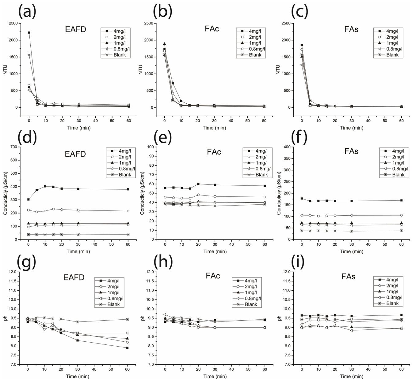
Fig. 2. Wastewater turbidity, NTU (a)–(c); electrical conductivity (d)–(f); and pH (g)–(i) as a function of time (min), using EAFD, FAc and FAs as coagulants, respectively (from left to right) at different dosages (mg/L). The blank sample measurements were conducted using only marble wastewater.
