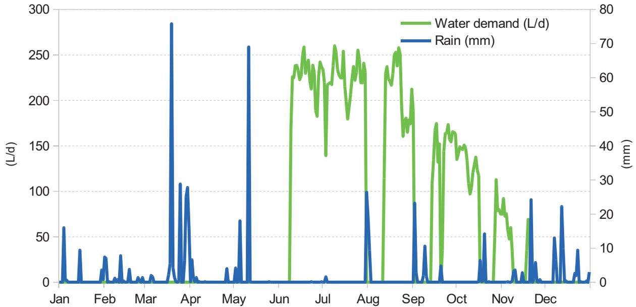
Fig. 6. Water required during 1999 (as estimated by UWOT) for irrigating the 50 m<sup>2</sup> green area of the case study and rainfall depth during the same period.
