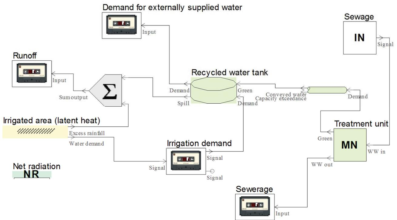
Fig. 4. Representation of the case study water network in UWOT.
