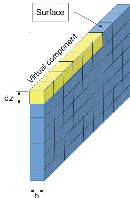
Fig. 2. Part of the Energy2D grid (up to the land surface) with the virtual component highlighted.
