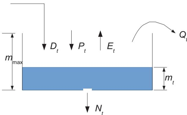
Fig. 1. Soil moisture model used in UWOT to estimate latent heat and water demand.
