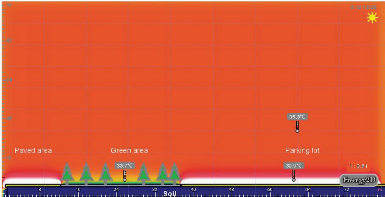
Fig. 7. Simulation of the heat fluxes and resulting temperatures.
