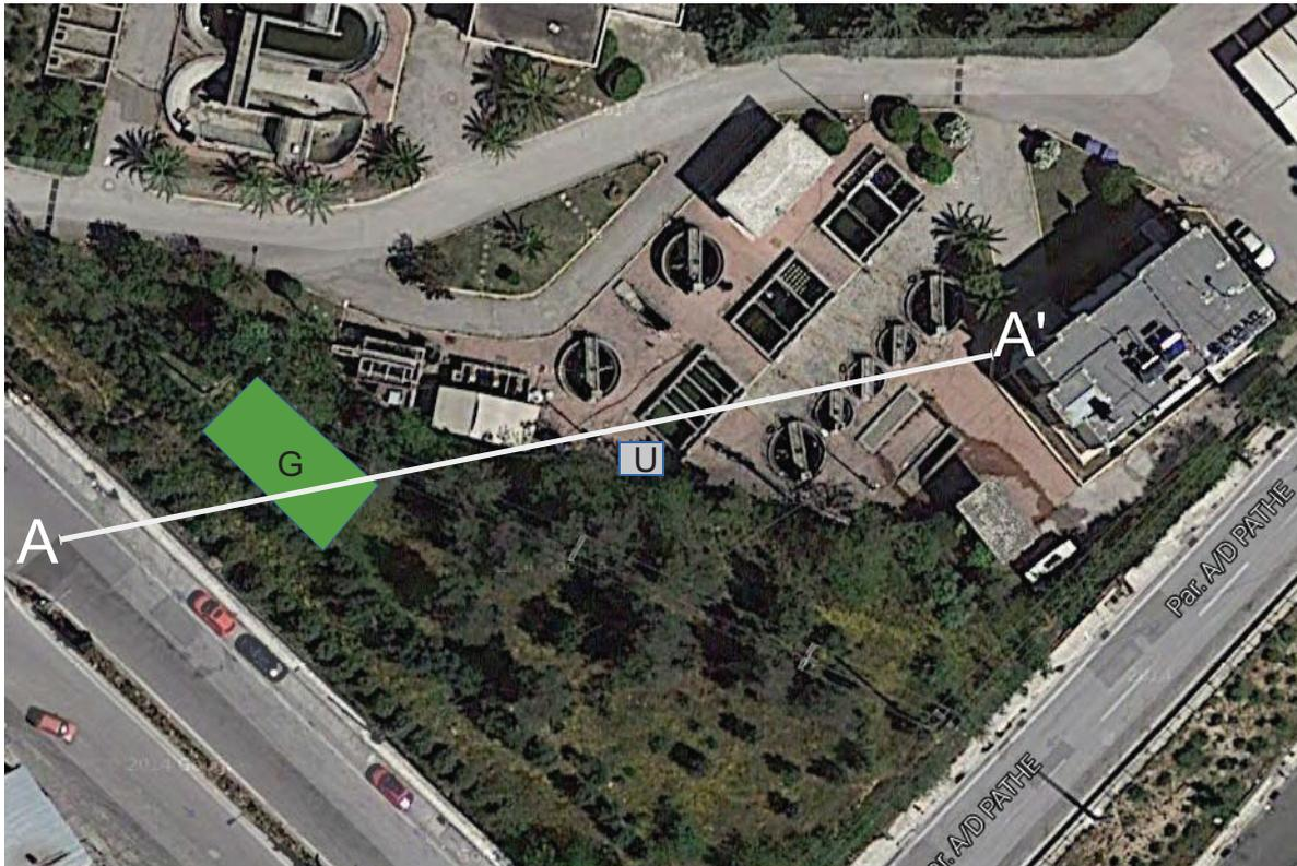
Fig. 3. The irrigated green area (marked with the green rectangle G) and the compact treatment unit (marked with the grey rectangle U). AA' line (80 m long) gives the axis along which the Energy2D simulation is performed.
