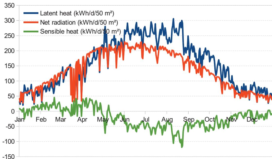
Fig. 5. Heat fluxes over the  $50 \text{ m}^2$  green area of the case study estimated by the UWOT simulation from 1 January 1999 to 31 December 1999.
