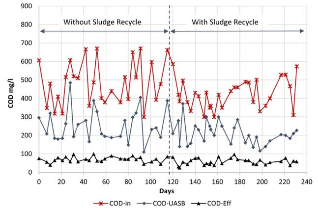
Fig. 2. COD values of raw wastewater, UASB effluent, and SBR effluent.
