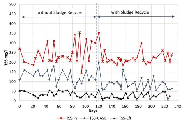
Fig. 3. TSS values of raw wastewater, UASB effluent, and SBR effluent.
