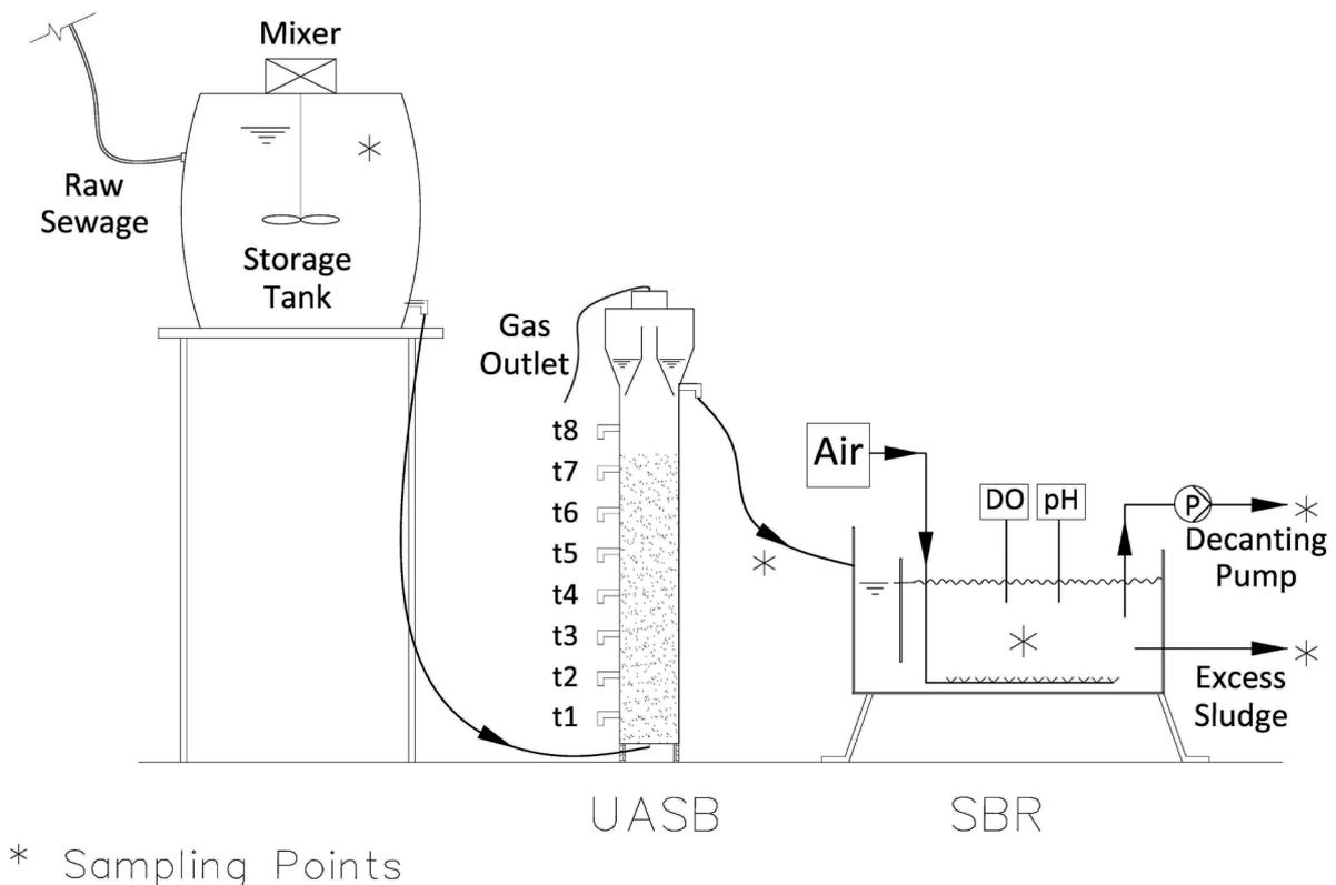
Fig. 1. Schematic of the combined UASB and cSBR system.
