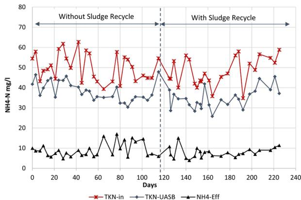
Fig. 4. TKN and  $NH_4-N$  values of raw wastewater raw wastewater, UASB effluent, and SBR effluent.
