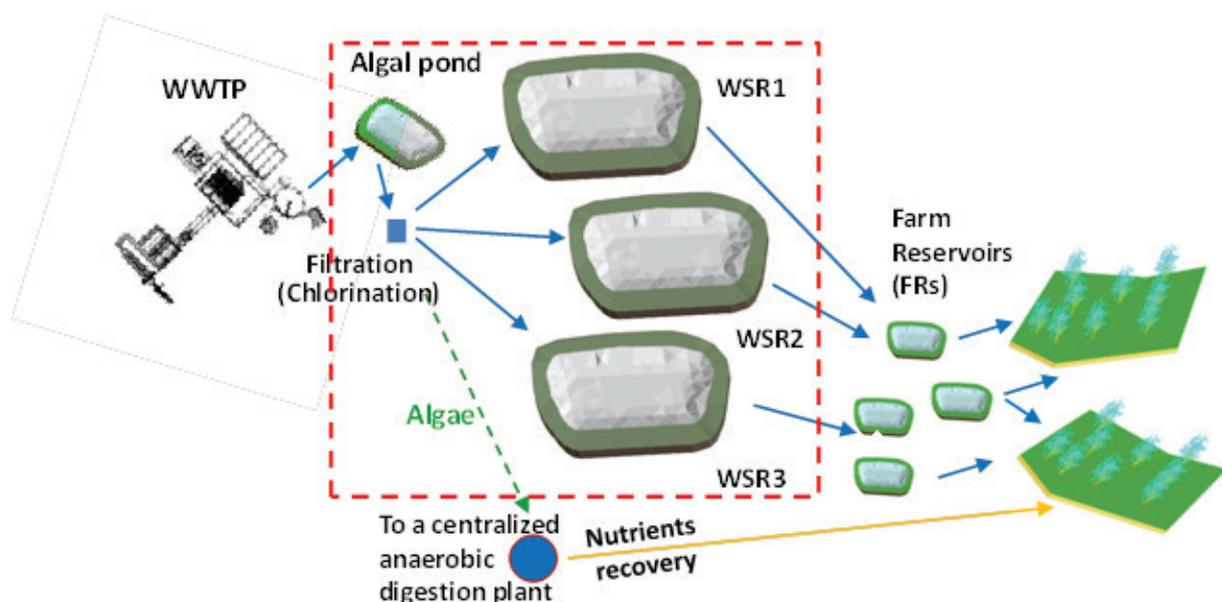
Fig. 1. Sketch of the wastewater reuse system with the proposed modifications (dashed rectangle).
