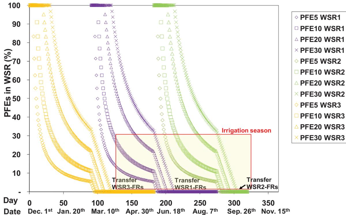
Fig. 5. Simulated variability, over the year, of the  $PFE_n$  values in the three WSRs calculated for a different number of days ( $n = 5, 10, 20$  and  $30$ ).
