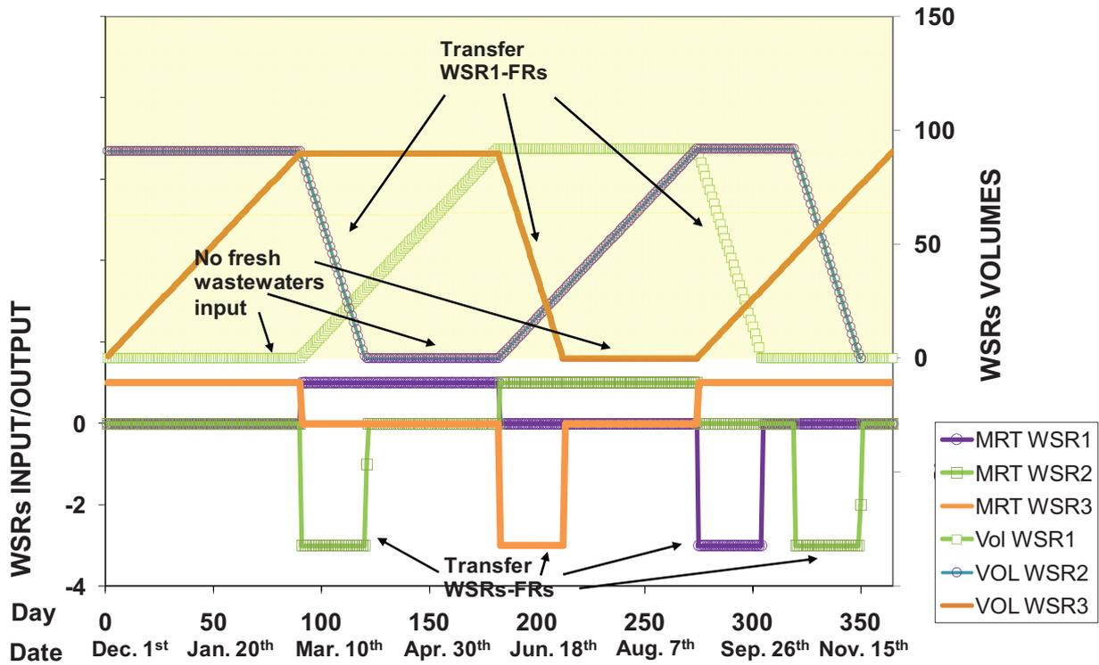
Fig. 3. Variations in the volume and inflow–outflow over the year in the WSRs (the unit volume is equal to 1 d of mean flow).
