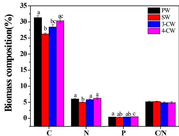
Fig. 2. Biomass composition of carbon (C, %), nitrogen (N, %), phosphorus (P, %) and C/N in biomass after cultured in different wastewaters for four continuous growth cycles (24 d). Different small letters on the bars indicate significant difference ( $p < 0.05$ ).
