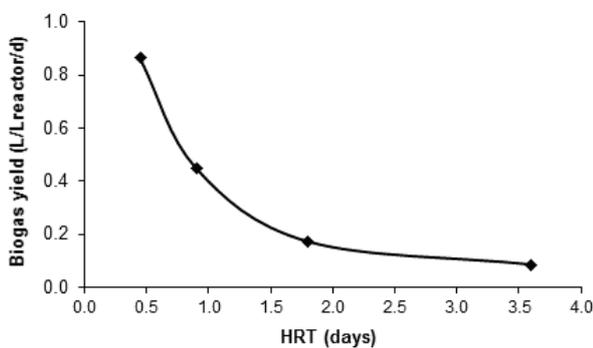
Fig. 7. Biogas yield during AD treatment of HTC effluent at 180°C for 90 min with AD hydraulic retention times of 0.45–3.6 d.
