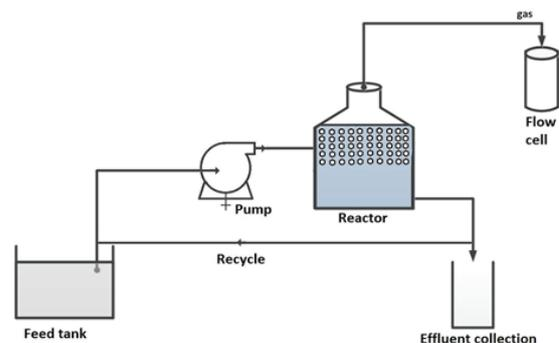
Fig. 1. Schematic of the anaerobic digestion process operated in a warm room (37°C).
