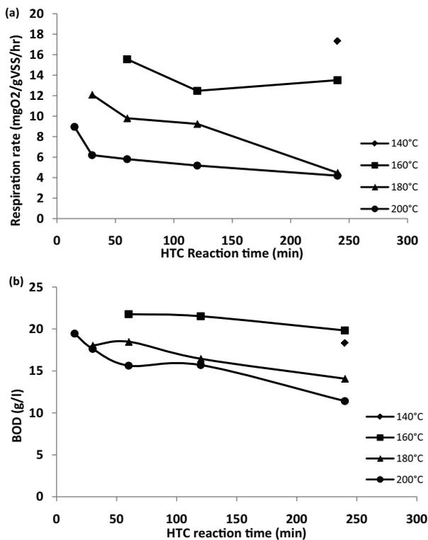
Fig. 5. (a) Respiration rate and (b) BOD of liquid filtrates after HTC treatment at 140°C–200°C and 30–240 min.
