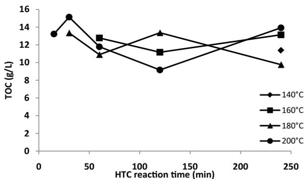
Fig. 4. Total organic carbon (TOC) of liquid filtrates after 140°C–200°C and 30–240 min HTC treatment.
