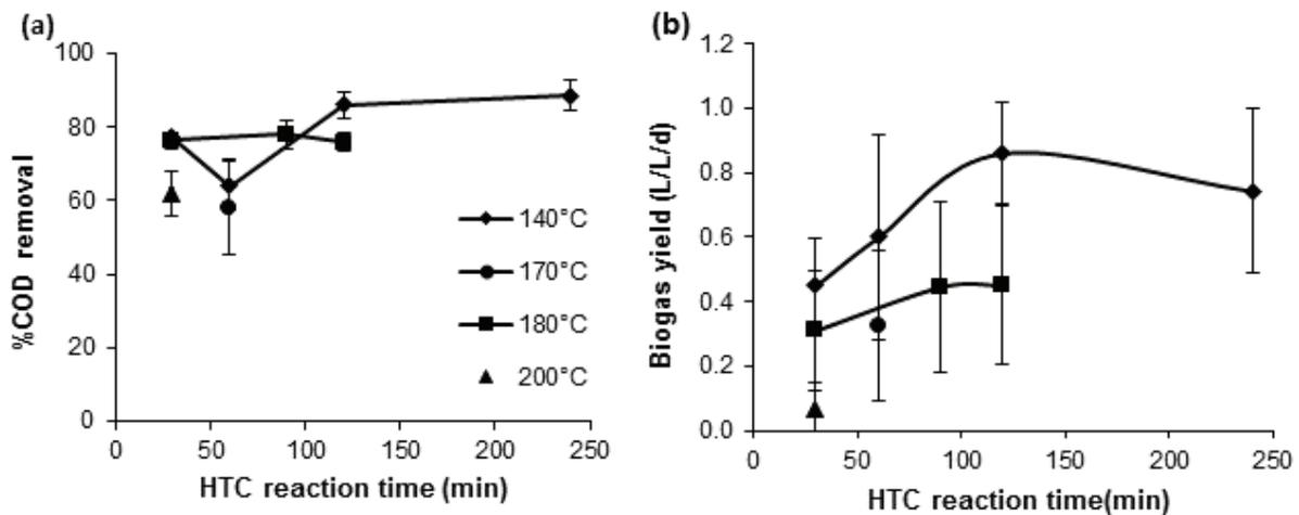
Fig. 3. Results of (a) COD removal and (b) biogas yield, during AD treatment of HTC effluent carbonised at 140°C–200°C for 30–240 min.
