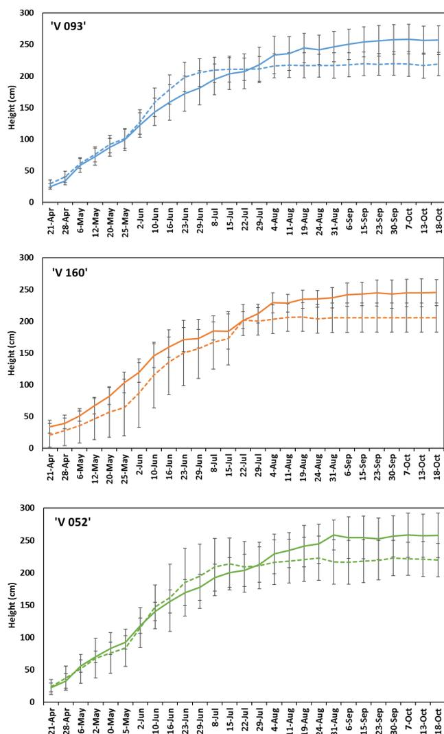
Fig. 3. Height of three willow clones 'V 093', 'V 160', and 'V 052' in pilot evapotranspirative willow system (solid line) and controls (dashed line) during first vegetation season. Means and standard deviations are given ( $N = 9$  and  $6$  for test and control willows, respectively).
