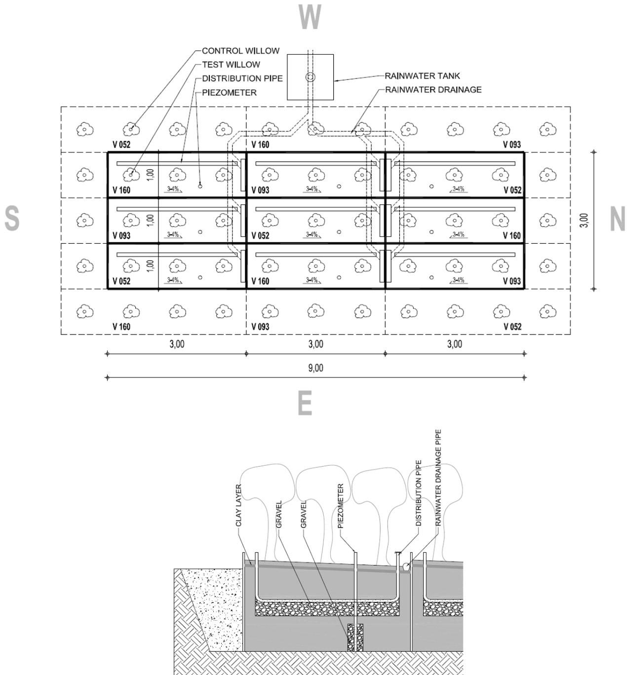
Fig. 1. Design of a pilot evapotranspirative willow system consisting of nine impermeable test beds and control willows planted around the pilot system (top-down view of the whole system and a cross-section of a test bed; units in meters).
