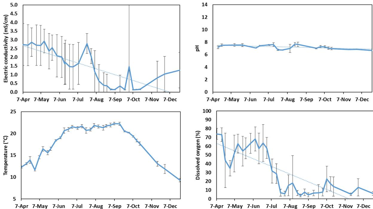
Fig. 2. Electric conductivity, pH, temperature and dissolved oxygen in all nine test beds of a pilot evapotranspirative willow system through vegetation season (mean  $\pm$  SD;  $N = 32$ ).
