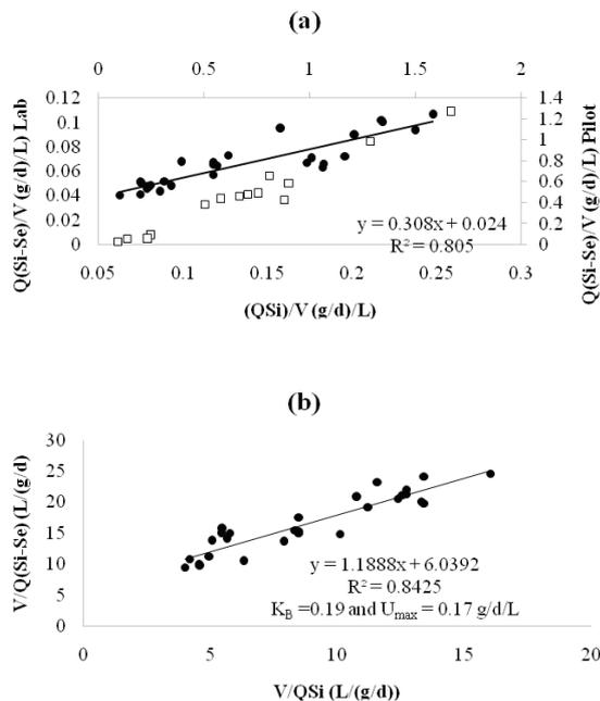
Fig. 5. Relationship between (a) organic removal rate vs. organic loading rate and (b) Stover–Kincannon kinetic model in lab-scale (●) and pilot-scale (□) of PBR.
