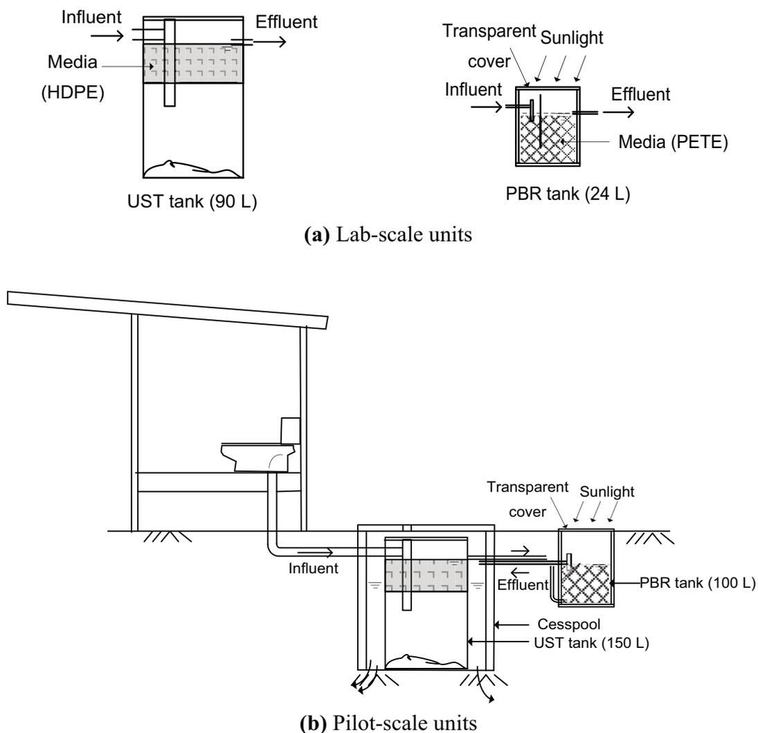
Fig. 1. Setup of (a) lab-scale and (b) pilot-scale experiments.
