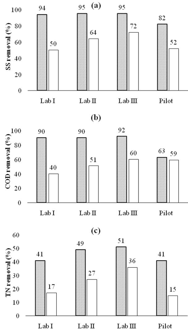
Fig. 3. Percentage of (a) SS, (b) COD and (c) TN removal efficiencies by UST (■) and PBR (□).
