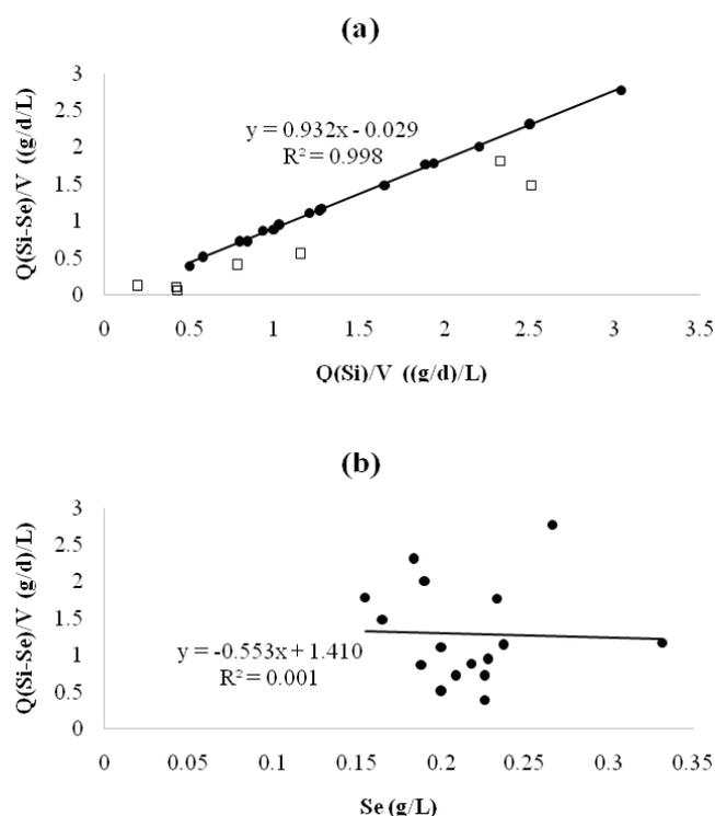
Fig. 4. Relationship between (a) organic removal rate (ORR) vs. organic loading rate (OLR) and (b) first-order rate for organic removal in lab-scale (●) and pilot-scale (□) of UST.
