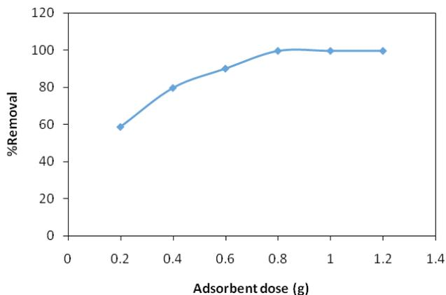
Fig. 3. Effect of the sorbent amount (the conditions used in this figure were the same of that of Fig. 2, except for sorbent amount).
