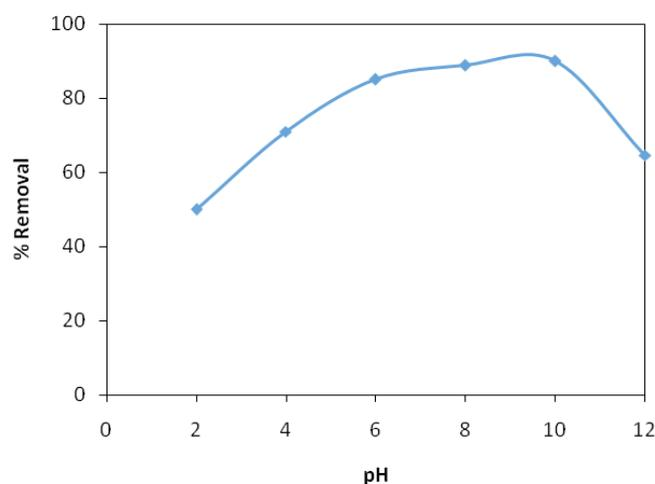
Fig. 2. Effect of pH on the adsorption of Cd(II) ions onto *Prunus avium* (with the following conditions: 50 mL of 150.0  $\text{mg L}^{-1}$  concentration of Cd(II), contact time of 60 min, agitation speed of 400 rpm and sorbent dose of 0.5 g).
