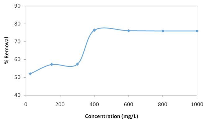
Fig. 5. Effect of the concentration on the % removal of Cd(II) ions by *Prunus avium* stems.
