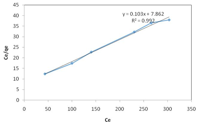
Fig. 7. Langmuir isotherm for Cd(II) biosorption onto *Prunus avium* stems.
