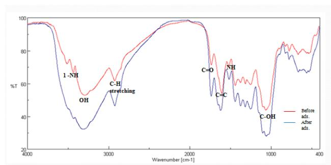
Fig. 1. FT-IR spectrum of *Prunus avium* stems before and after adsorption.
