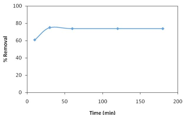
Fig. 4. Effect of contact time on adsorption of Cd(II) ions onto *Prunus avium* (conditions were the same as in Fig. 2, except for contact time).
