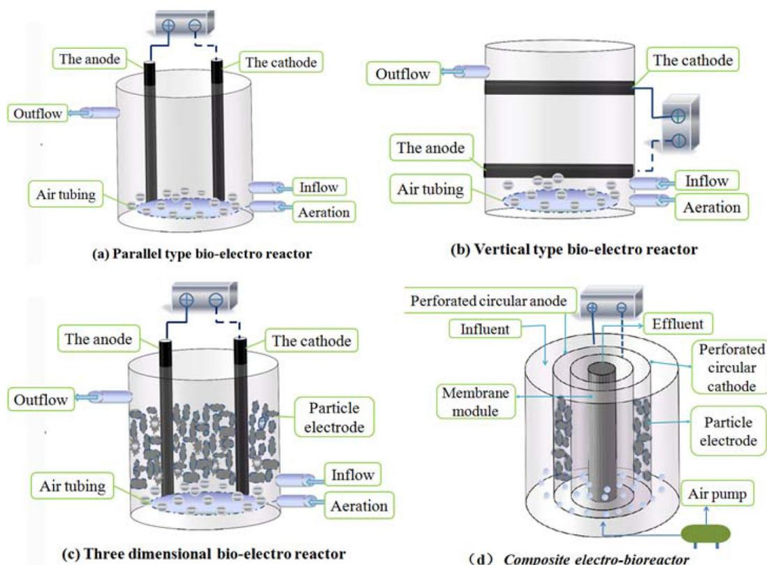
Fig. 1. Some typical structure of EBCP.
