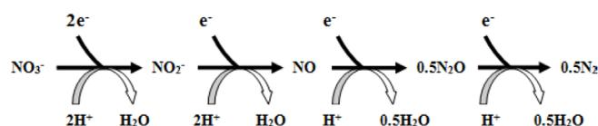
Fig. 2. Reaction process of  $\text{NO}_3^-$  conversion to  $\text{N}_2$ .
