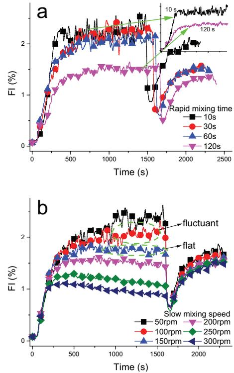
Fig. 7. Flocs growth, breakage and regrowth. Influence of rapid mixing duration (a) and slow mixing speed (b).
