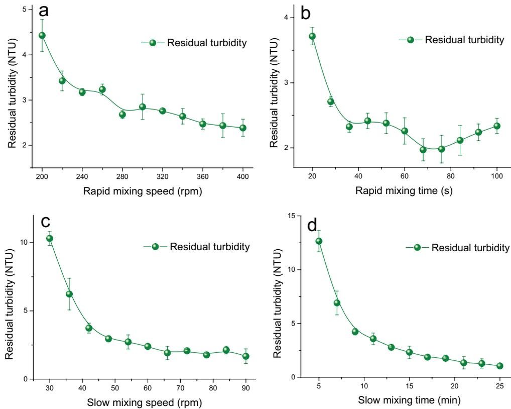
Fig. 4. Influence of single factor on turbidity removal: rapid mixing speed (a); rapid mixing time (b); slow mixing speed (c) and slow mixing time (d).
