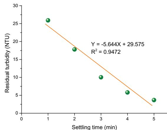
Fig. 2. Correlation between residual turbidity and settling time.
