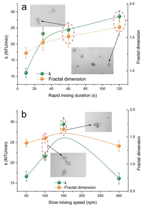
Fig. 8. Relationship between flocs settleability and fractal dimension. Influence of rapid mixing duration (a) and slow mixing speed (b). ‘k’, calculated as the variation ratio of residual turbidity, was selected as the representative for floc settleability. Representative flocs images were selected from images of online capture using a CCD camera.
