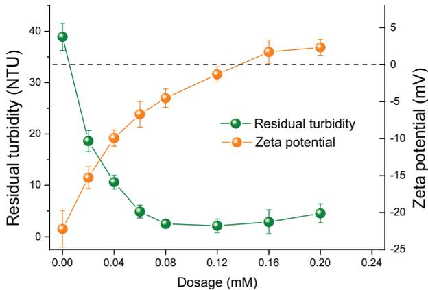
Fig. 3. Influence of coagulant dosage on residual turbidity and zeta potential.
