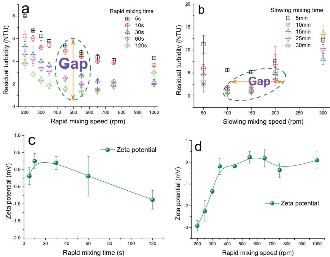
Fig. 5. Influence of mixing conditions in coagulation (a) and flocculation (b) on turbidity removal. Influence of rapid mixing time (c) and speed (d) on zeta potential.
