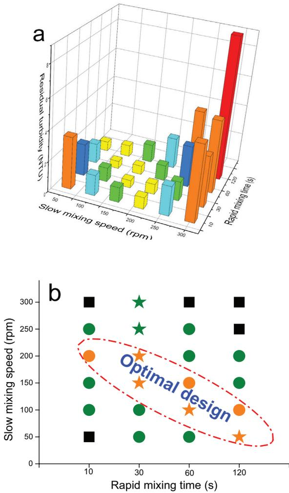
Fig. 6. Interaction between coagulation and flocculation on turbidity removal (a); optimal operational design of coagulation–flocculation process (b). Residual turbidity level: orange < 0.8 NTU, 0.8 NTU < green < 3.0 NTU and black > 3.0 NTU.
