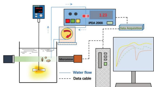
Fig. 1. A schematic diagram of online floc formation monitor system.
